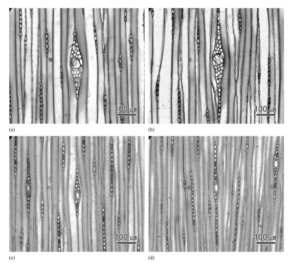
Figure 1. Representative optical micrographs of the tangential sections in *Pinus koraiensis* (a-b) and *Larix kaempferi* (c-d). (a, c) Near the pith; (b, d) near the bark.
