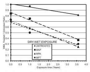
Figure 9. Treated/untreated WML ratio for samples exposed under DRY-WET conditions.
