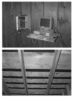
Figure 2. Interior view of exposure units showing data acquisition system (upper) and exposure portals (lower) for plywood samples.
