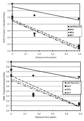
Figure 4. Comparison of treated/untreated MOR (upper) and WML (lower) ratios in the laboratory study.
