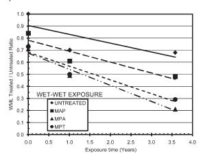
Figure 10. Ratio of treated/untreated WML for wet samples exposed under wet conditions.
