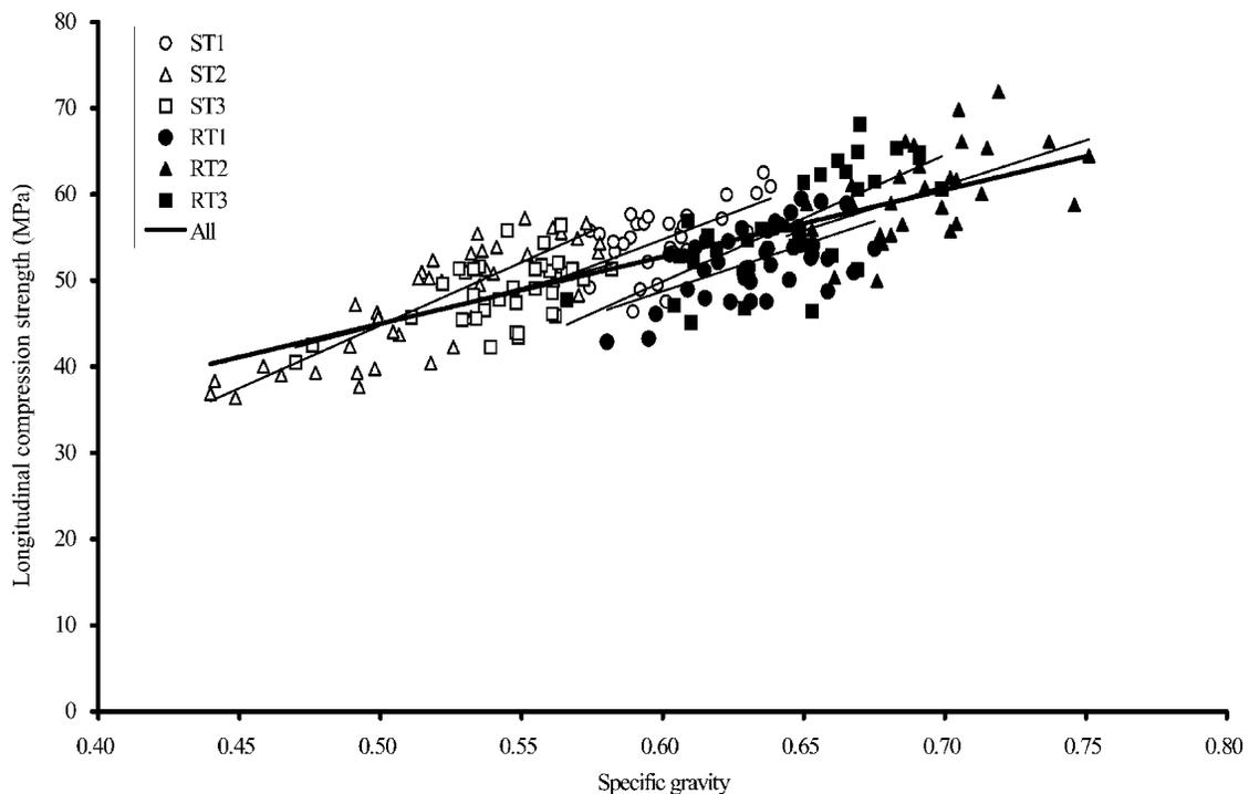
FIG. 4 Relationship between specific gravity and longitudinal compression strength.
