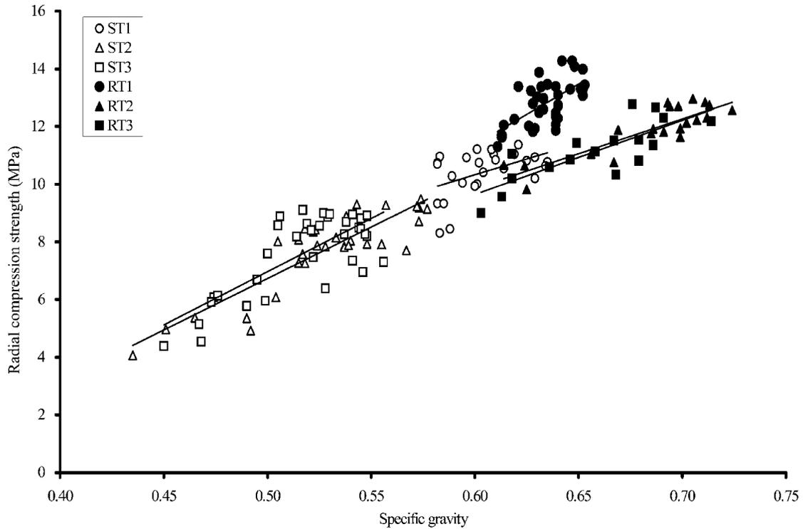
FIG. 5. Relationship between specific gravity and radial compression strength.
