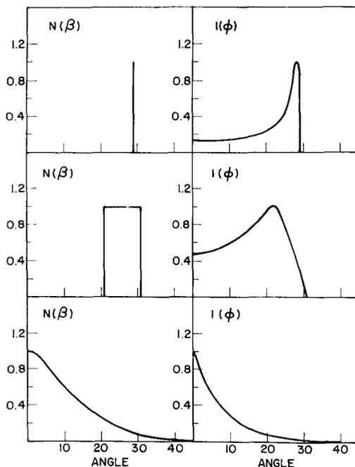
FIG. 5. Comparison between several fibril angle distribution functions  $N(\beta)$  and the corresponding X-ray intensity functions  $I(\phi)$  for circular fibers.
