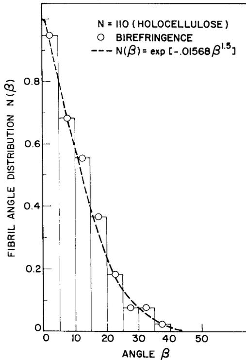
FIG. 2. Fibril angle distribution function as a function of angle for a black spruce sample, as obtained from the microscope reflectance method.
