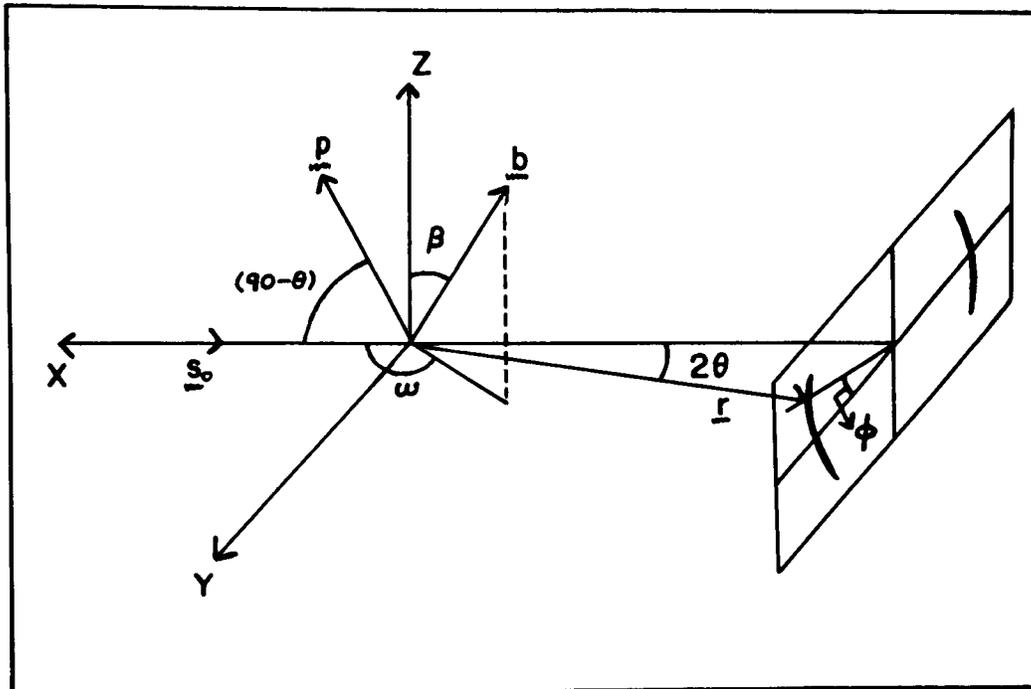
FIG. 1. Schematic representation of the diffraction geometry.
