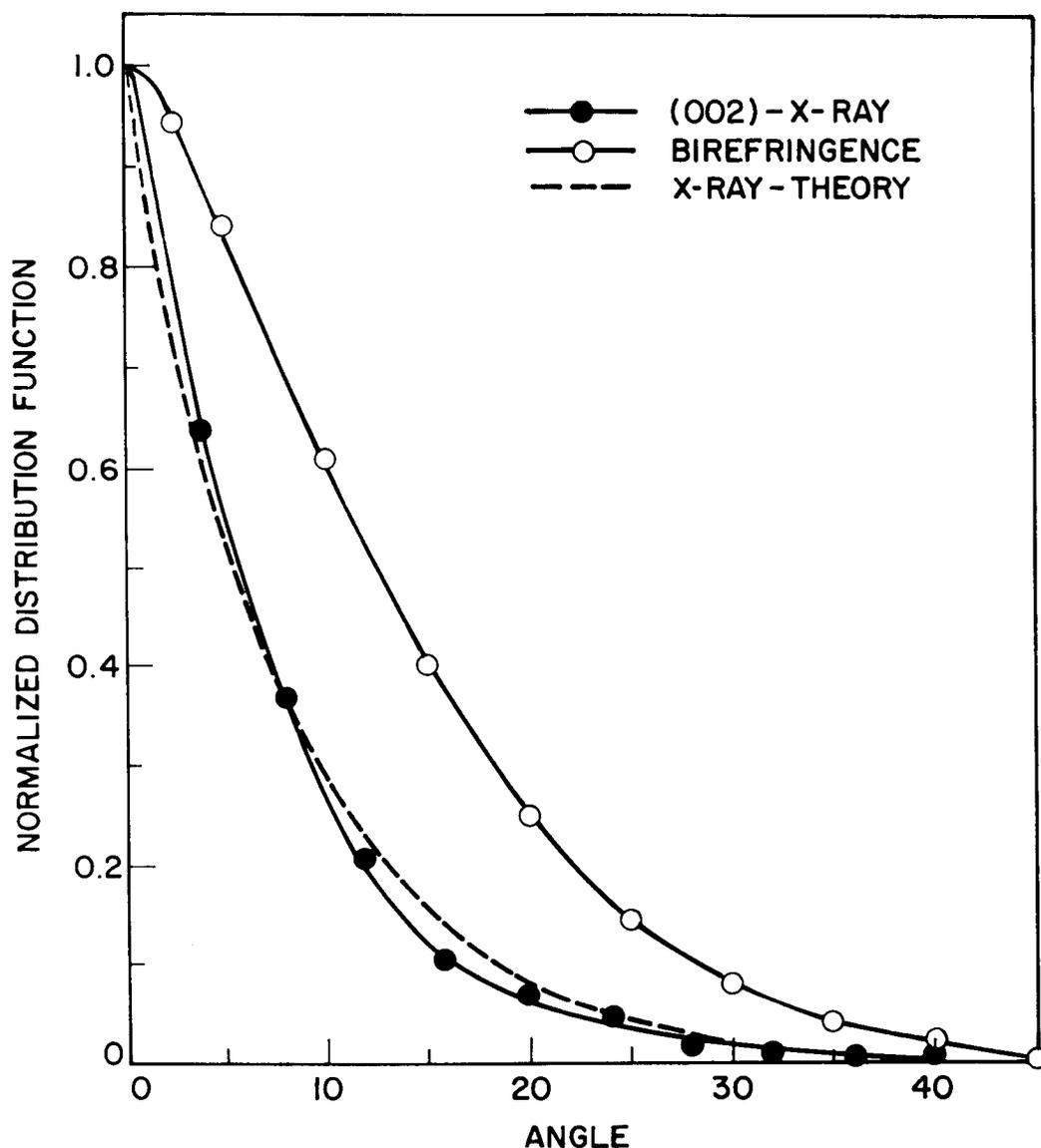
FIG. 4. Comparison between the measured fibril angle distribution function as obtained by the reflectance method and the X-ray intensity data of the (002) plane for a wood sample. The dotted line is the theoretical X-ray intensity curve.
