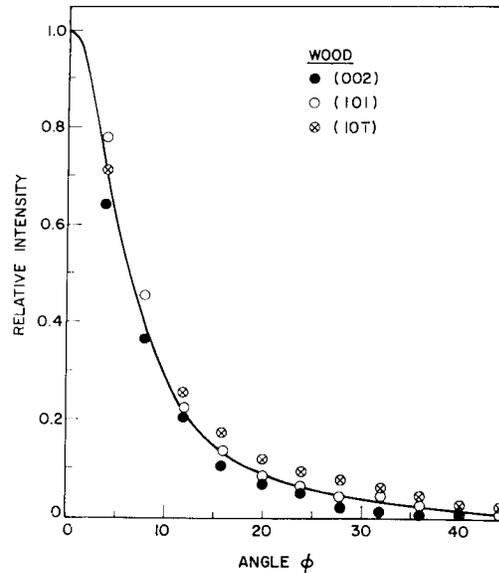
FIG. 3. Experimental distribution of intensity as a function of angle for the (002), (101), and (10 $\bar{1}$ ) planes of a wood sample.
