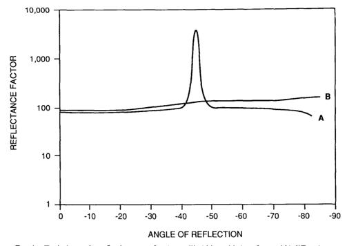
FIG. 4. Typical specular reflection curve for a) metallic (shiny white) surface and b) diffuse (matte white) surface. Adapted from Hunter and Harold (1987, p. 43).
