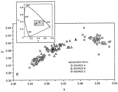
FIG. 5. CIE chromaticity diagram plotted with color coordinates for various wood species, as reported in the references cited in the accompanying text section. Samples measured with the same CIE standard source (A, B, or C) occupy relatively small areas that, though slightly overlapping, are distinct.
