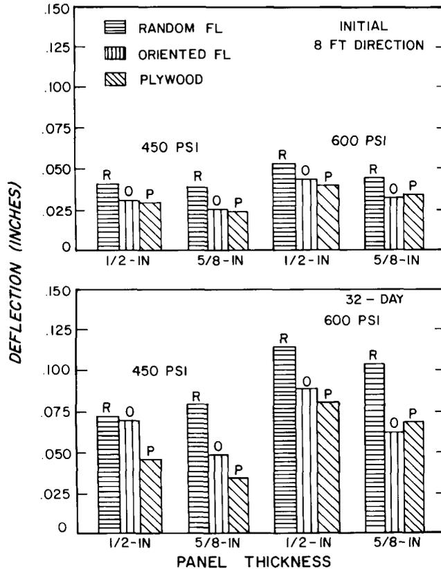
FIG. 5. Relationship between deflection of plywood, random flakeboard, and oriented flakeboard, 1/2-inch and 5/8-inch thick, when initially loaded (top) and after 32 days of a continuous load (bottom) at 450 psi and 600 psi bending stress on small bending specimens obtained from the 8-foot panel direction.
