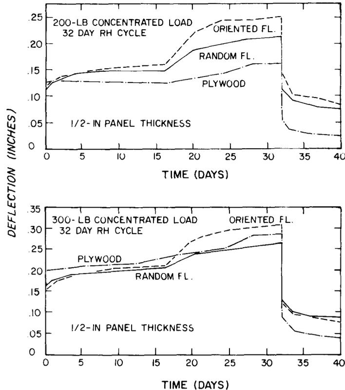
FIG. 7. Deflection versus time relationship for 1/2-inch-thick random flakeboard, oriented flakeboard, and plywood when subjected to 200-lb and 300-lb concentrated loads and 16 days of 50% RH plus 16 days of 85% RH.
