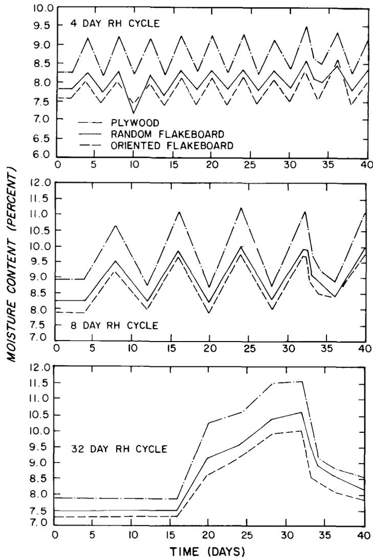
FIG. 4. Moisture content fluctuation for plywood, random flakeboard, and oriented flakeboard when subjected to a cyclic 50–85% relative humidity change every 4, 8, and 32 days.
