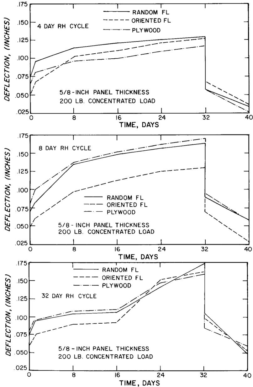
FIG. 8. Deflection versus time relationship for  $\frac{5}{8}$ -inch-thick random flakeboard, oriented flakeboard, and plywood when subjected to 200-lb concentrated load and a 4-, 8-, and 32-day relative humidity cycle of 50 to 85%.
