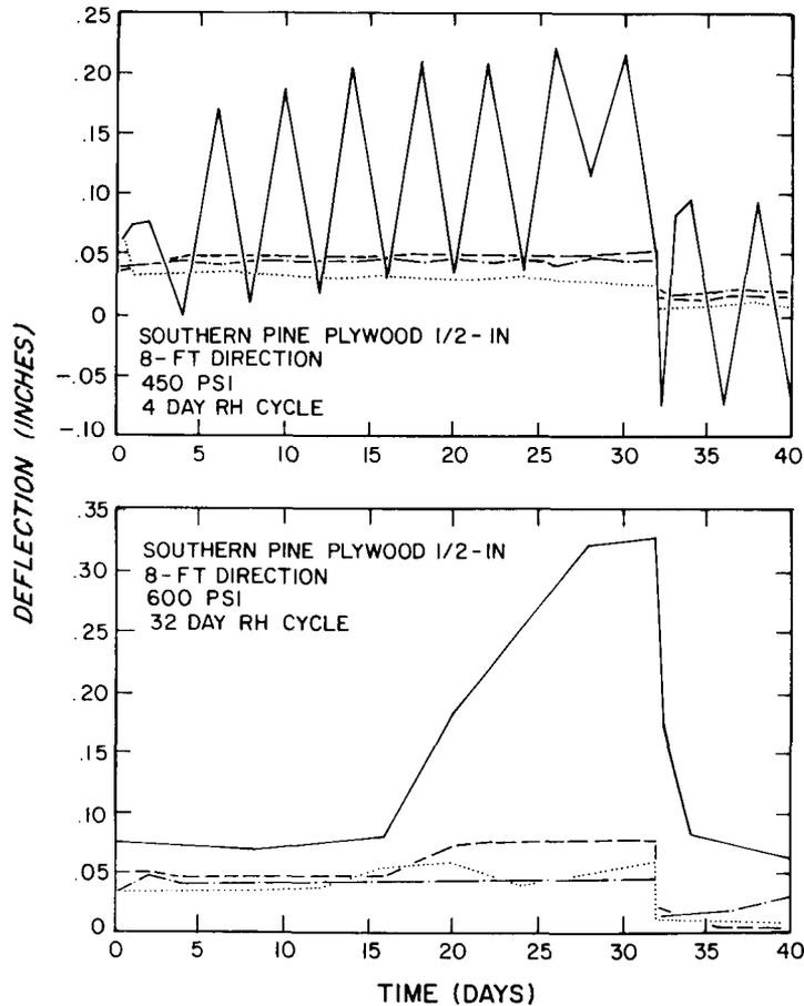
FIG. 3. Deflection curves for four different southern pine plywood specimens subjected to 450 psi (top) and 600 psi (bottom) stresses.
