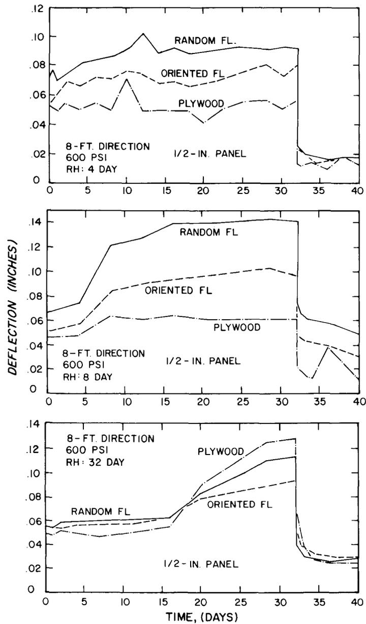
FIG. 6. Deflection versus time relationship for 1/2-inch-thick random flakeboard, oriented flakeboard, and plywood specimens obtained from the 8-foot panel direction and subjected to 600 psi continuous stress for 32 days under a 4-, 8-, and 32-day relative humidity cycle of 50 to 85%.
