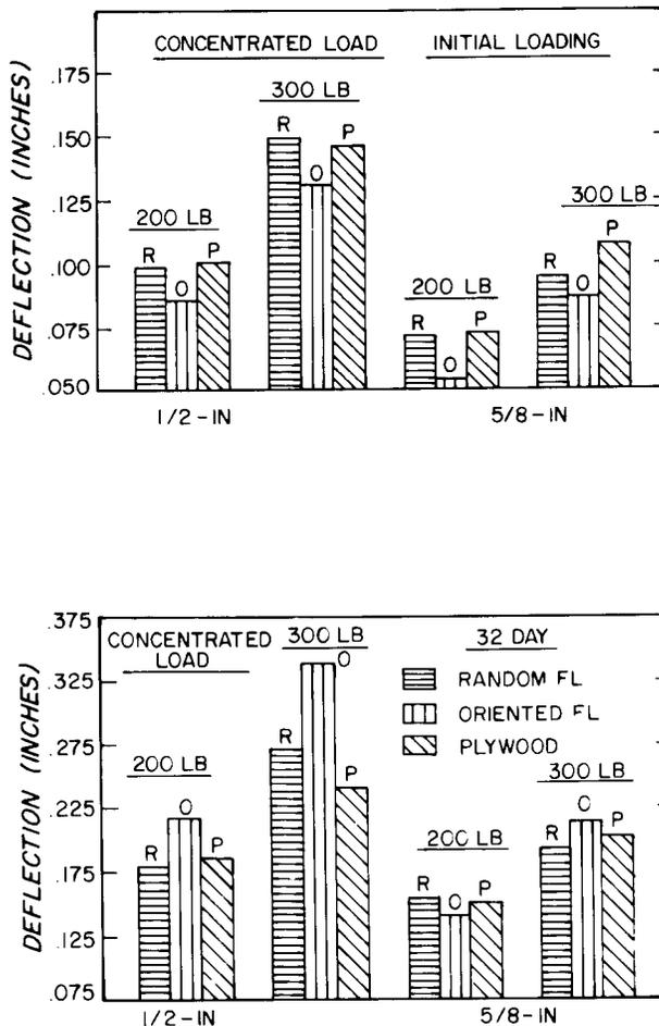
FIG. 9. Initial and 32-day deflection relationship for 1/2- and 5/8-inch-thick random flakeboard, oriented flakeboard, and plywood when subjected to 200- and 300-lb concentrated loads.
