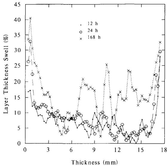
FIG. 4. Thickness swell distributions of the oriented strandboard after three water soak exposure times.
