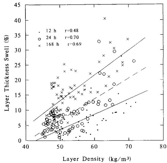
FIG. 7. The relationship between layer density and layer thickness swell of the oriented strandboard.
