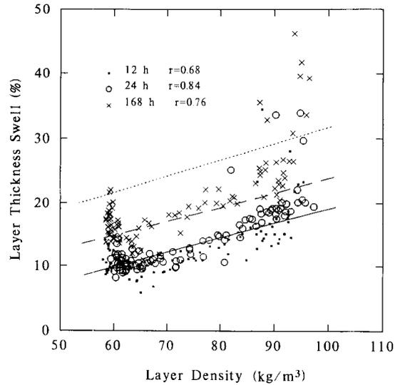
FIG. 9. The relationship between layer density and layer thickness swell of the particleboard.
