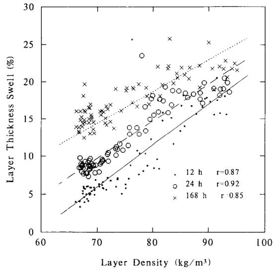
FIG. 3. The relationship between layer density and layer thickness swell of the medium density fiberboard.
