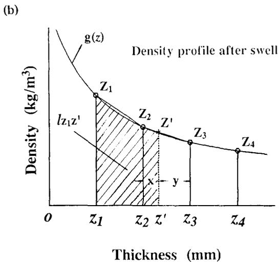
FIG. 1. A schematic showing the procedures of estimating the thickness swell distribution in wood composites.
