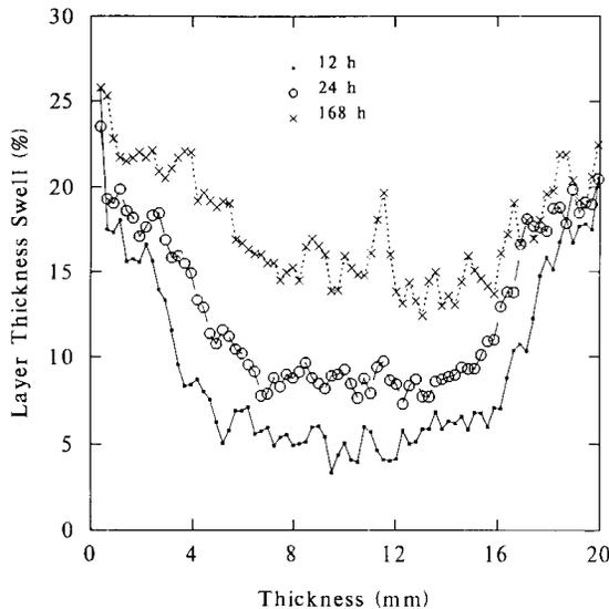
FIG. 2. Thickness swell distributions of the medium density fiberboard after three water soak exposure times.
