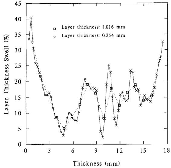
FIG. 6. Thickness swell distributions of the oriented strandboard determined at two resolution thicknesses.
