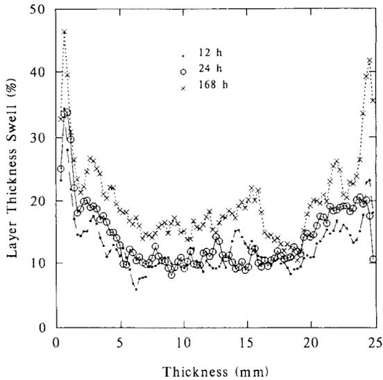
FIG. 8. Thickness swell distribution of the particleboard after three water soak exposure times.
