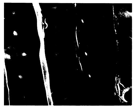
Fig. 6. Bordered pit structures of southern yellow pine on radial section (×1,000).
