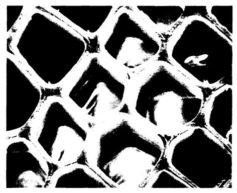
Fig. 2. Cross section of southern yellow pine ( $\times 1,000$ ).
