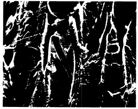
Fig. 10. Microchecks of cell wall of southern yellow pine at tangential section (latewood) after exposure to ultraviolet light for  $500 \text{ h} \ (\times 1,000)$ .
