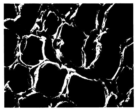
Fig. 3. Cross section of southern yellow pine exposed to ultraviolet light for 500 h (×1,000).
