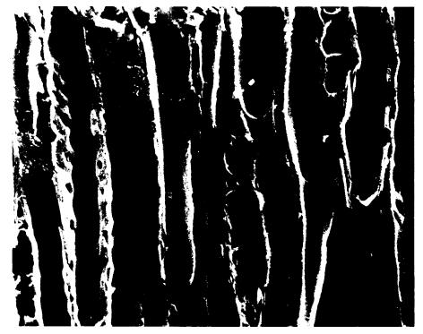
Fig. 15. Tangential section of southern yellow pine treated with 5% ferric chloride solution after exposure to ultraviolet light for 500 h ( $\times$ 1,000).
