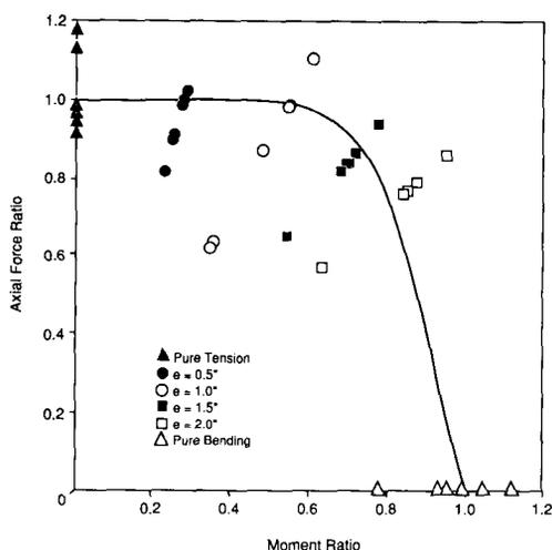
FIG. 10. Tension-bending interaction curve of tension splice joints.
