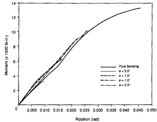
FIG. 6. Moment-rotation curves of tension splice joints under different loading conditions.
