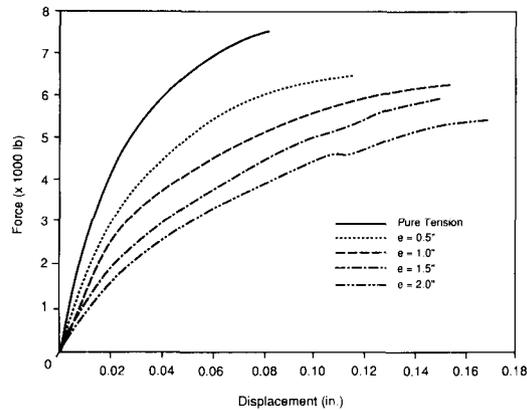
FIG. 4. Load-displacement curves of tension splice joints under different loading conditions.
