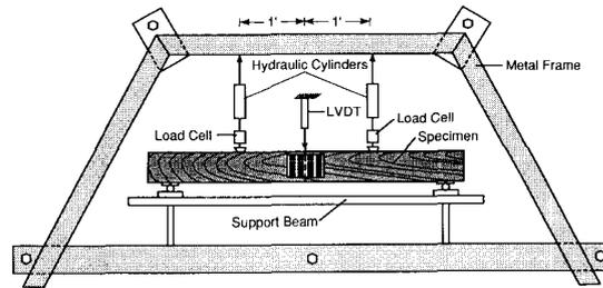
FIG. 2. Test frame with tension splice joint under pure bending loading.
