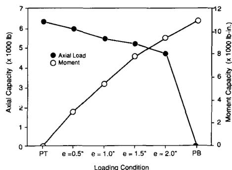
FIG. 9. Moment and axial capacities for different loading conditions.
