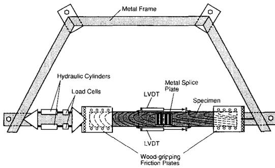
FIG. 1. Test frame with tension splice joint under axial tension loading.
