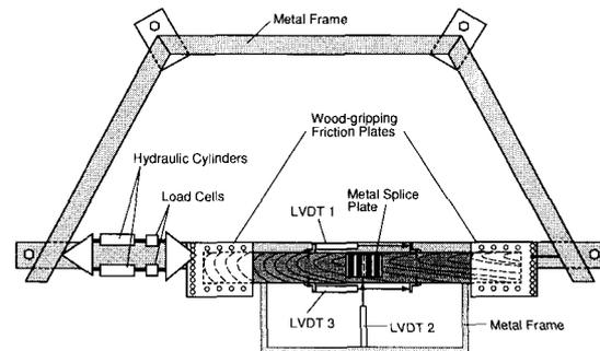
FIG. 3. Test frame with tension splice joint under combined (axial tension/bending) loading.
