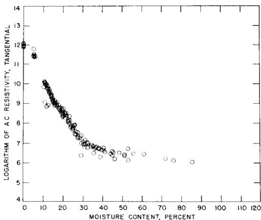
FIG. 7. Relation of the logarithm of tangential AC resistivity of western hemlock to moisture content.
