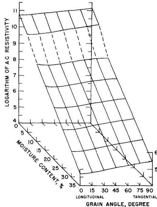
FIG. 14. Effect of grain orientation in LT-plane and moisture content on AC resistivity of western hemlock.
