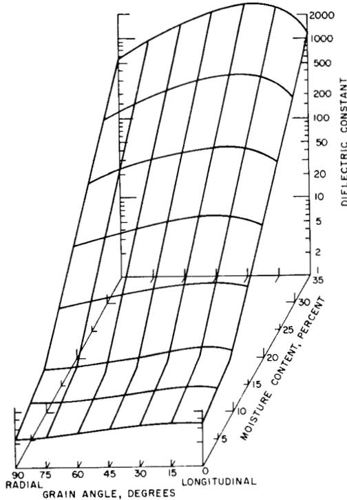
FIG. 10. Effect of grain orientation in LR-plane and moisture content on dielectric constant of western hemlock.
