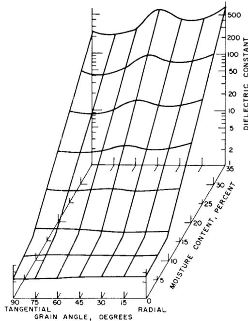
FIG. 12. Effect of growth-ring orientation in RT-plane and moisture content of western hemlock on its dielectric constant.
