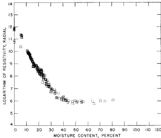
FIG. 6. Relation of the logarithm of radial AC resistivity of western hemlock to moisture content.
