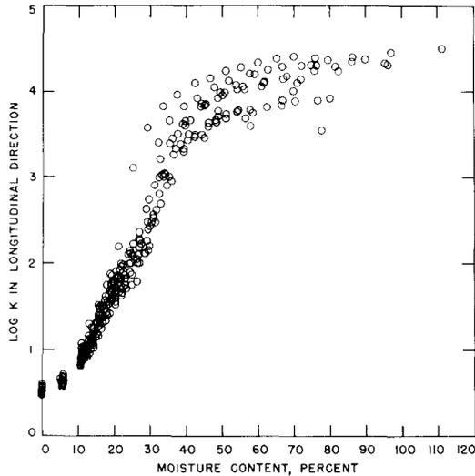
FIG. 2. Relation of the logarithm of longitudinal dielectric constant of western hemlock to moisture content.
