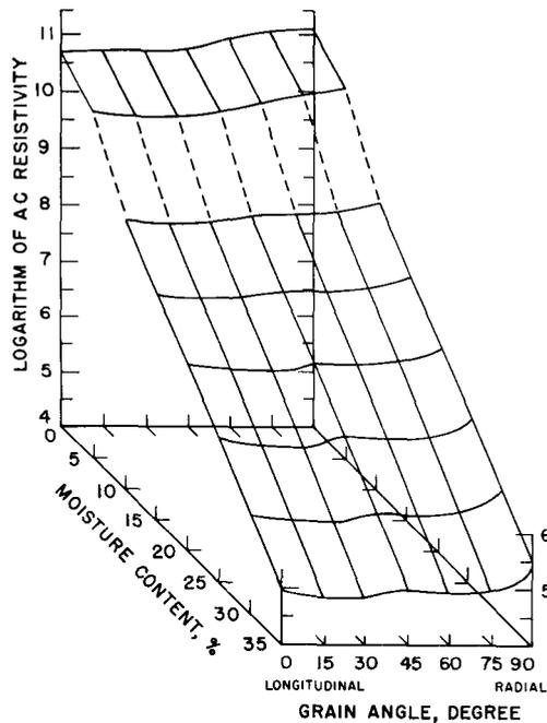
FIG. 13. Effect of grain orientation in LR-plane and moisture content on AC resistivity of western hemlock.
