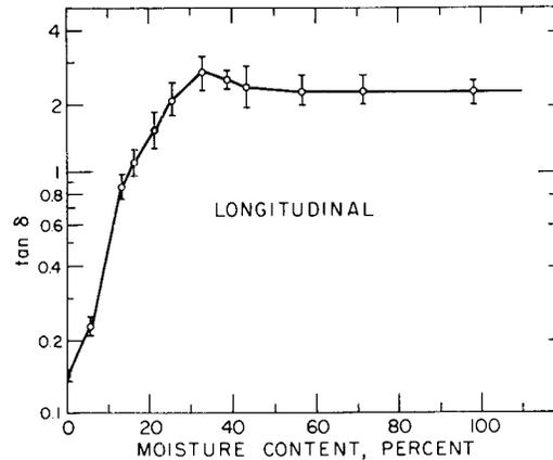
FIG. 8. Relation of the longitudinal loss tangent of western hemlock to moisture content.
