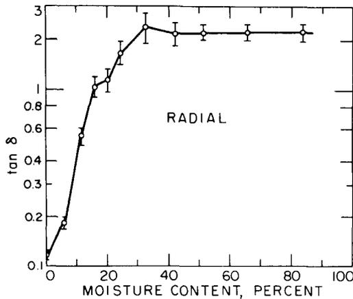
FIG. 9. Relation of the radial loss tangent of western hemlock to moisture content.
