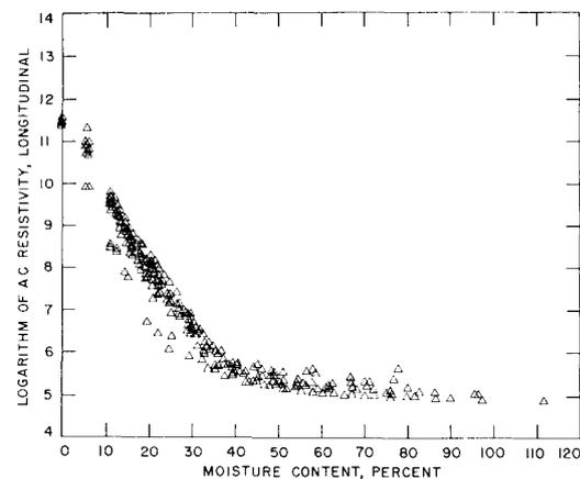
FIG. 5. Relation of the logarithm of longitudinal AC resistivity of western hemlock to moisture content.
