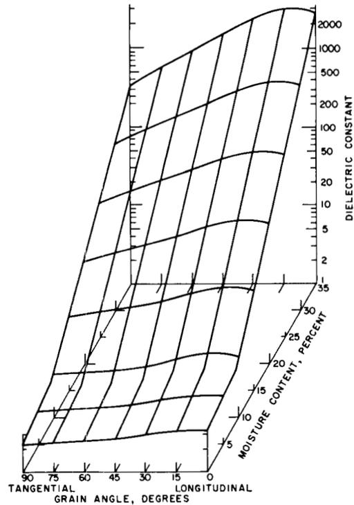
FIG. 11. Effect of grain orientation in LT-plane and moisture content on dielectric constant of western hemlock.
