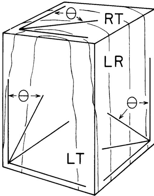
FIG. 1. Schematic presentation for cutting test specimens in various grain directions.
