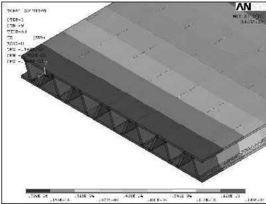
FIG. 7. Moisture deformation due to 86% RH.
