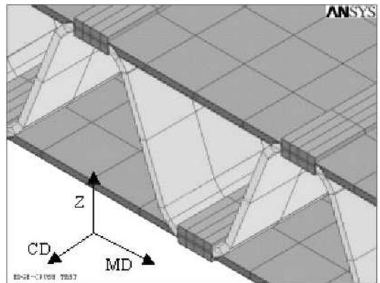
Fig. 2. FE geometry of the corrugated fiberboard.
