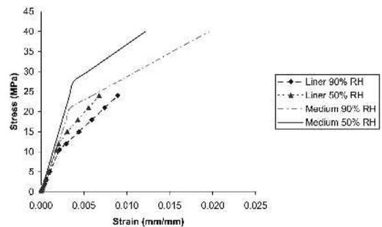
FIG. 1. Stress-strain curve for liner and medium.
