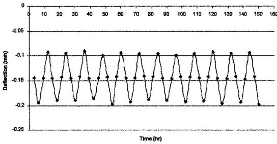
FIG. 5. FEA hydroexpansion response due to RH schedule.
