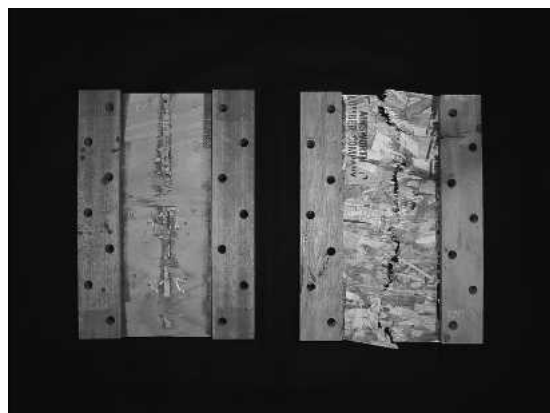
FIG. 3. Typical failure modes of PW (left) and OSB (right) specimens in static test.
