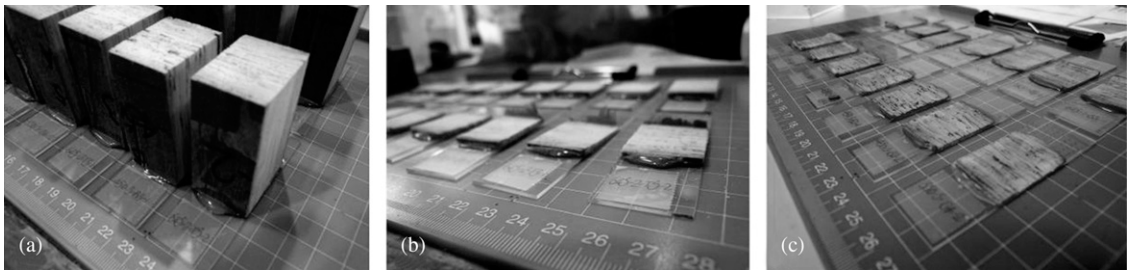
Figure 2. Slide preparation processes: (a) samples bonded to glass slide, (b) thick sections cut off with slides, and (c) finished slides after sanding.
