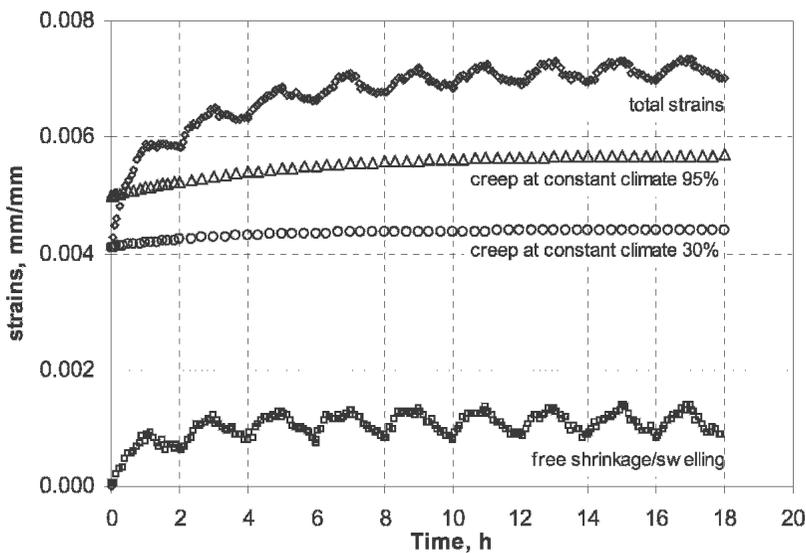
FIG. 3. Sample results from a set of tests at load level of 70% of green UTS.
