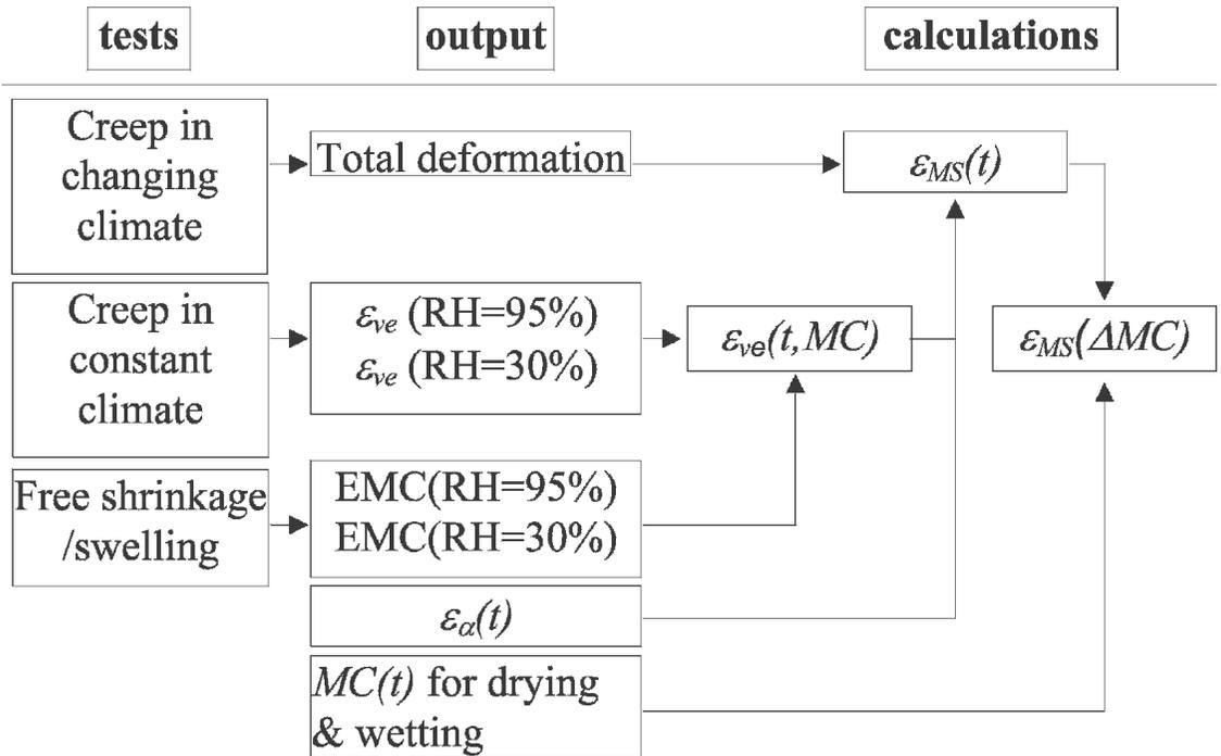
FIG. 2. Diagram summarizing three-step treatment of the experimental data. EMC is Equilibrium Moisture Content of wood at given ambient conditions (temperature and RH).
