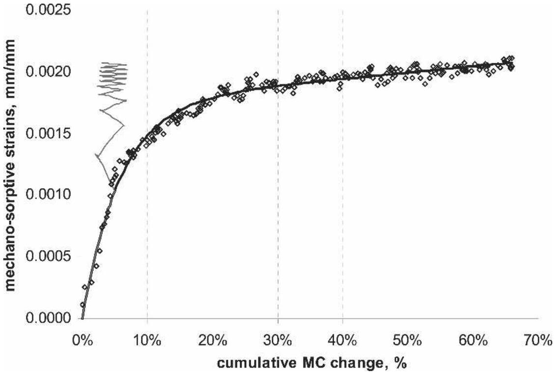
FIG. 4. An example of mechano-sorptive deformations presented in the MC domain (a) and cumulative moisture content change ( $\nu$ ) domain (b).
