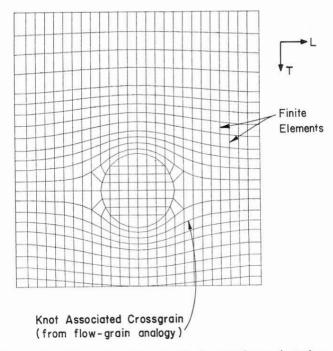
FIG. 1. Simulated grain pattern resulting from the flow-grain analogy.
