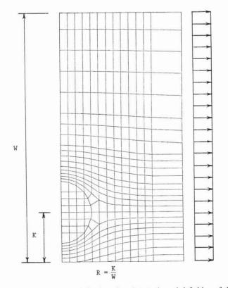
$F_{IG}.$  2. Example finite element mesh for knot location study and definition of the knot location ratio, R.
