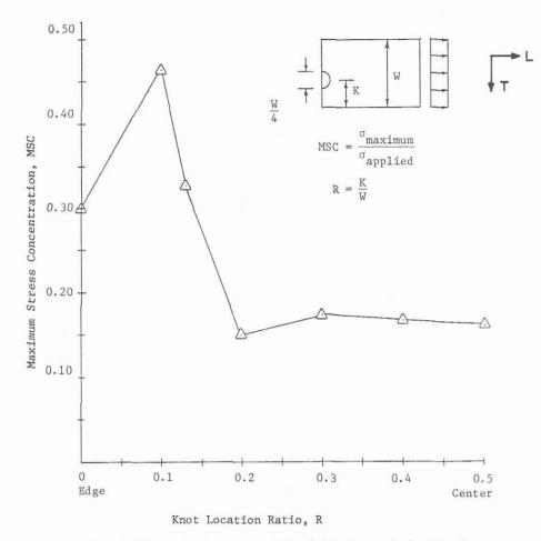
FIG. 4. Transverse stress concentration factors for varying knot location.
