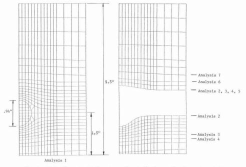
FIG. 6. Finite element mesh for segment B and effective sections for each analysis.
