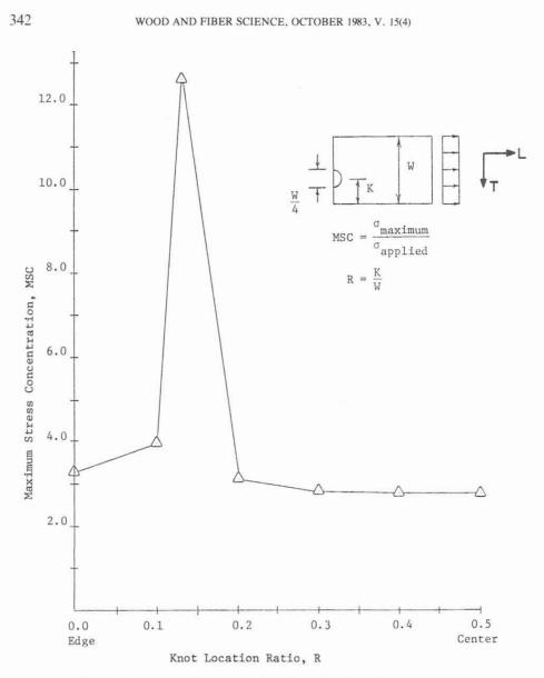
FIG. 3. Longitudinal stress concentration factors for varying knot location.
