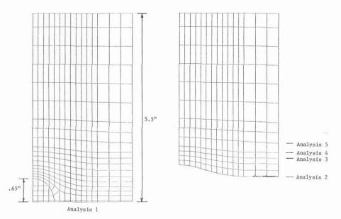
FIG. 5. Finite element mesh for segment A and effective sections for each analysis.
