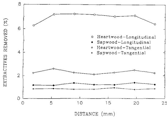
FIG. 2. Average extractive distribution profiles of southern pine heartwood and sapwood in the longitudinal and tangential directions at Extractive Stage A.
