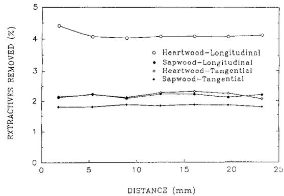
FIG. 3. Average extractive distribution profiles of southern pine heartwood and sapwood in the longitudinal and tangential directions at Extractive Stage B.
