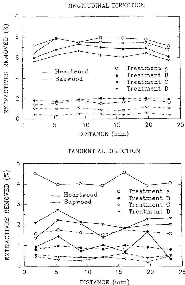
FIG. 4. Comparison of extractive distribution profiles of southern pine by four treatments at Extractive Stage A. Treatment A—control, Treatment B—steaming in green condition for 1 h at 100°C. Treatment C—steaming in green condition for 5 h at 100°C, Treatment D—hot-water soaking for 10 h at 70°C.
