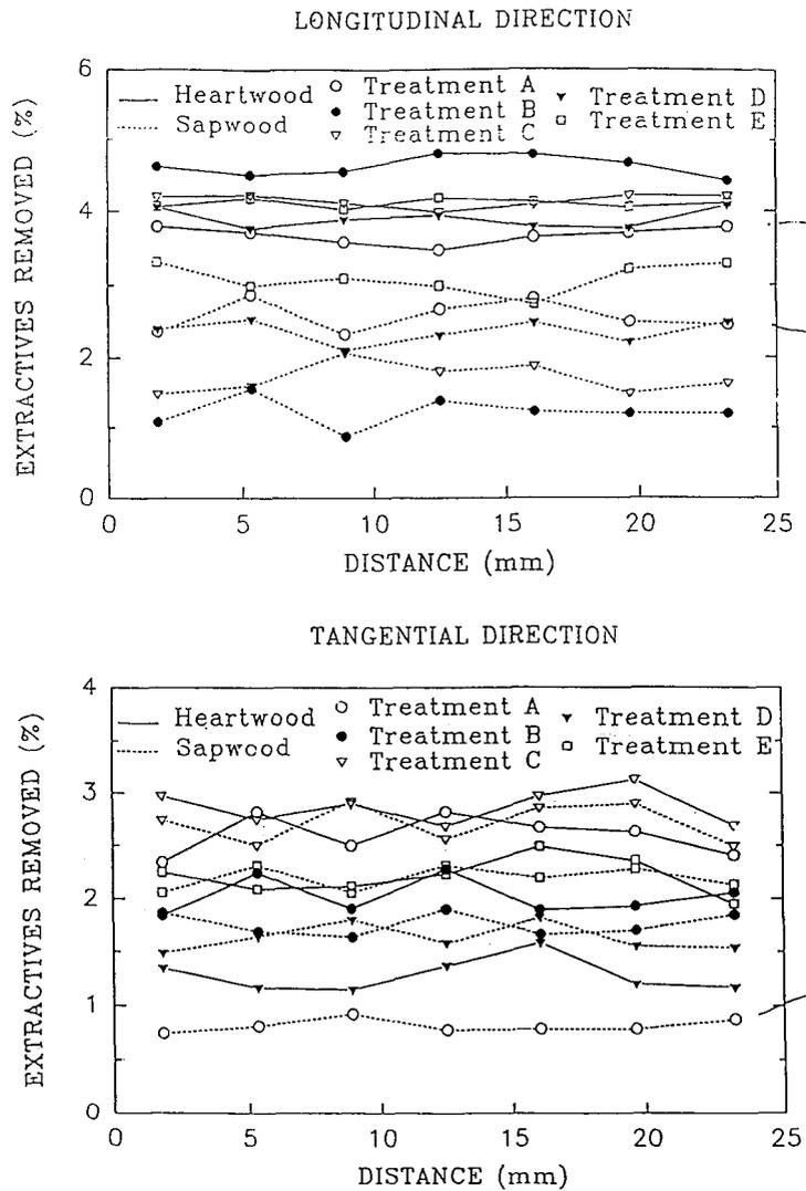
FIG. 5. Comparison of extractive distribution profiles of southern pine by five treatments at Extractive Stage B. Treatment A—control, Treatment B—steaming in green condition for 1 hour at 100° C, Treatment C—steaming in green condition for 5 hours at 100° C, Treatment D—hot-water soaking for 10 hours at 70° C, Treatment E—steaming at moisture content near the fiber saturation point for 1 hour at 100° C.
