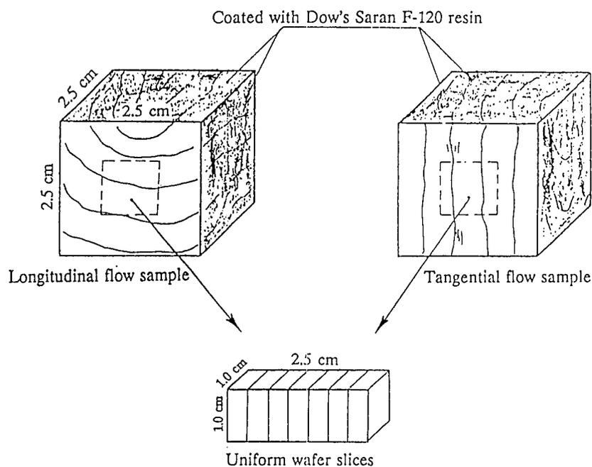
FIG. 1. Cutting scheme of extractive distribution profile samples.
