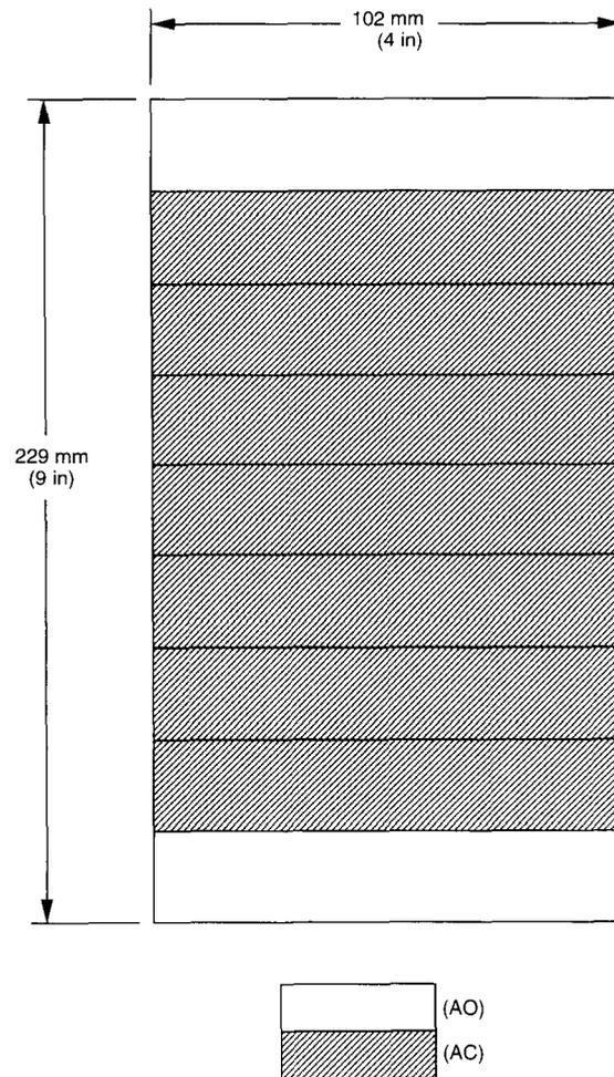
FIG. 1. Layup design for Combination A hardwood glulam.
