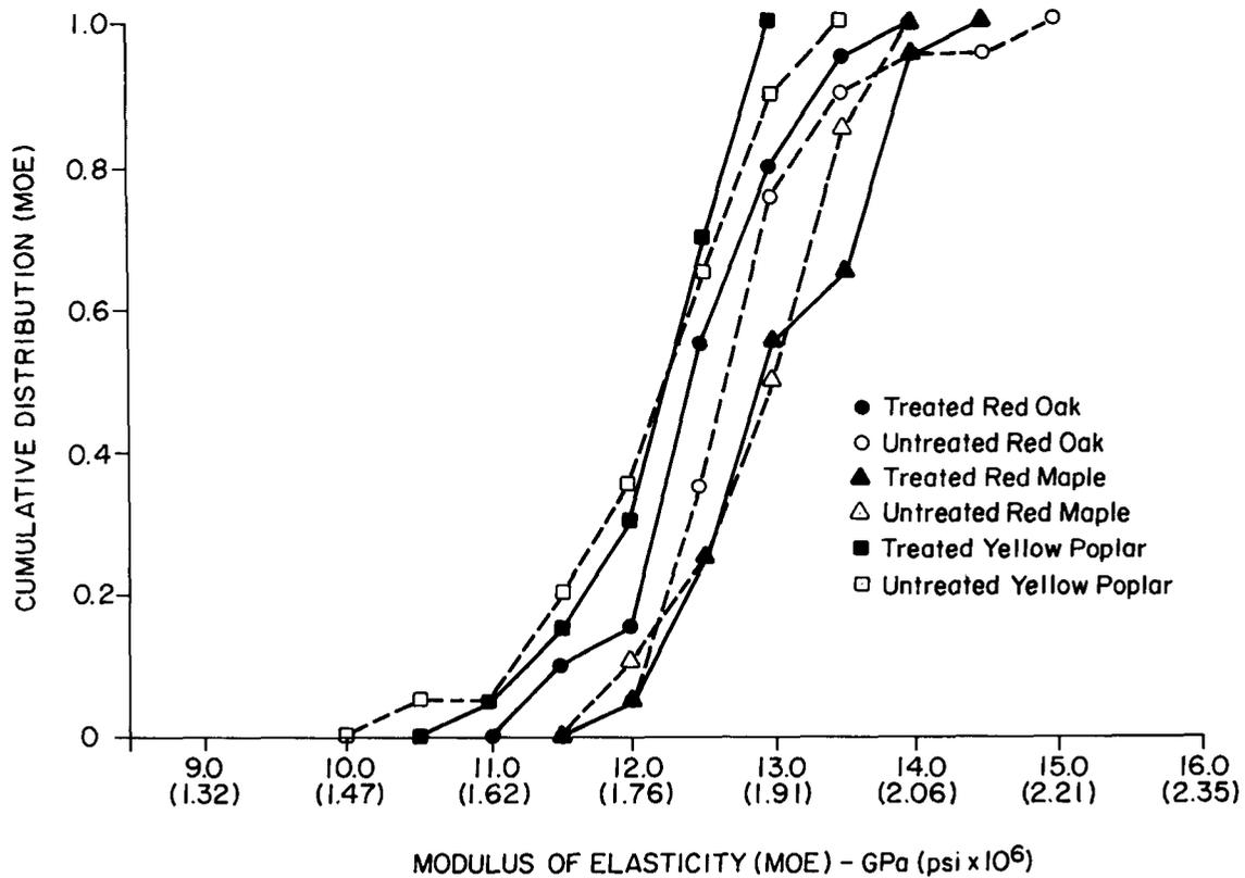
FIG. 5. Cumulative distributions of modulus of elasticity for treated and untreated red oak, red maple, and yellow poplar Combination A glulam beams.
