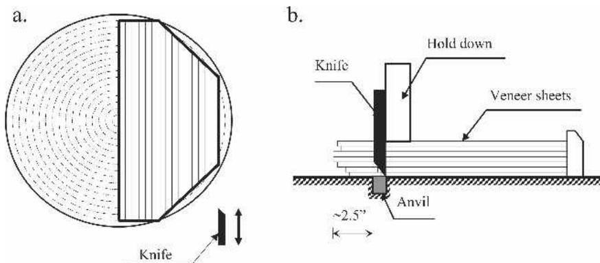
FIG. 1. Schematic of the decorative veneer manufacturing process. a.—Configuration of slicing. b.—The clipping operation.
