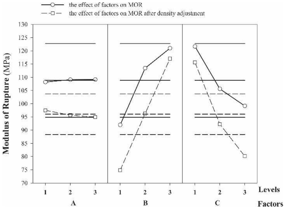
FIG. 6. Effect of factors on the modulus of rupture. Original and adjusted predictions are compared. Horizontal lines represent mean values and  $\pm 2$  standard errors.
