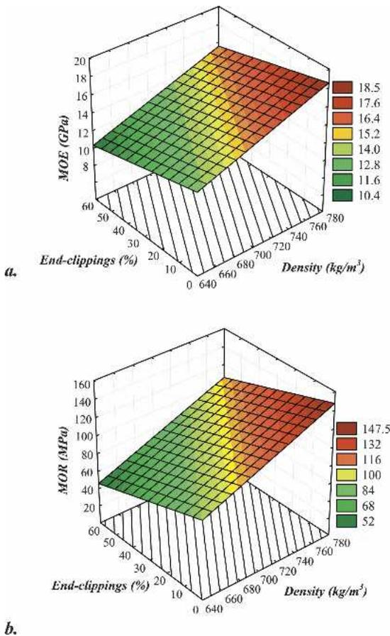
FIG. 7. Response surfaces predicting the expected mechanical properties as a function of factors B and C at fixed 8% resin content level. a. – Response surface of modulus of elasticity. b. – Response surface of modulus of rupture.
