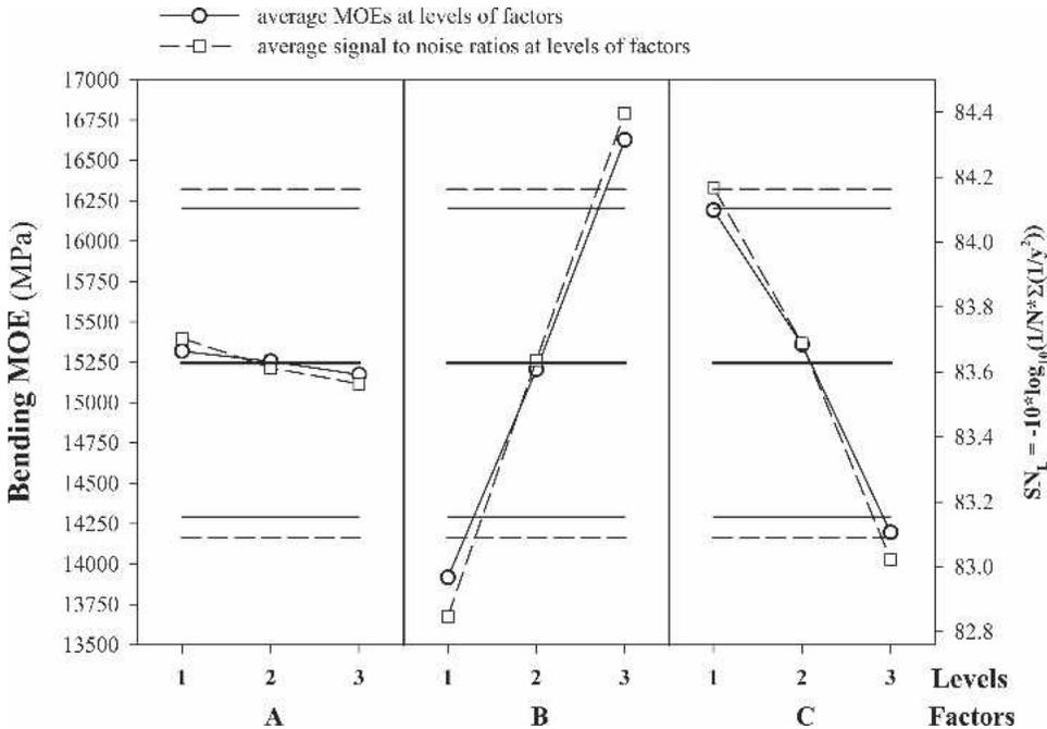
FIG. 5. Effect of factors on the modulus of elasticity. The predictions by mean values and SN<sub>L</sub> ratios are compared. Horizontal lines represent mean values and ± 2 standard errors.
