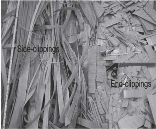
FIG. 2. Typical clipping residues generated by face veneer manufacture.
