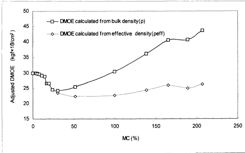
FIG. 7. Relationships between the corrected DMOE and MC in the radial direction.
