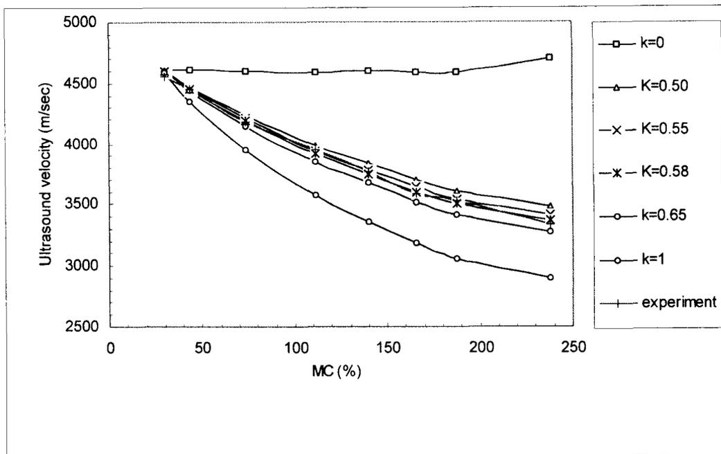
FIG. 9. Relationships between moisture content and velocity for ultrasonic wave to calculating the optimum value of the mobility of free water for the longitudinal specimens.
