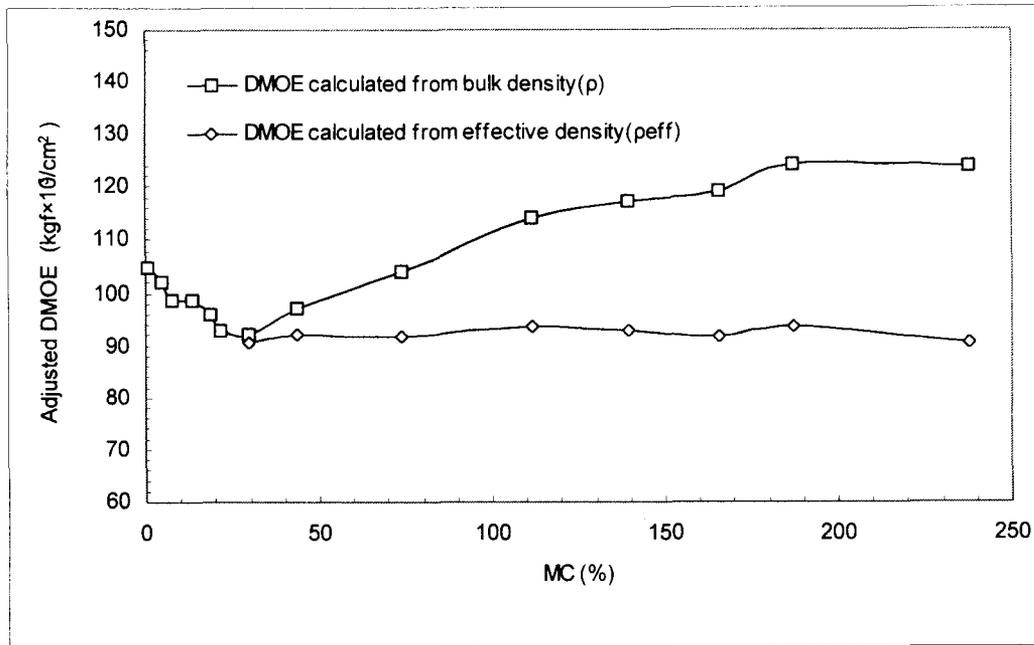
FIG. 6. Relationships between the corrected DMOE and MC in the longitudinal direction.
