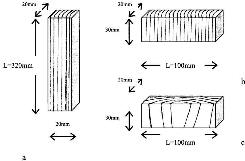
FIG. 1. Dimensions of specimens. a: for longitudinal transmission; b: for radial transmission; c: for tangential transmission; L: direction of measurement.
