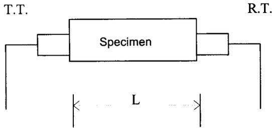
FIG. 2. Measuring method for ultrasonic velocity and dynamic modulus of elasticity of wood specimen. L: length of specimen; T.T.: transmitting transducer; R.T.: receiving transducer.
