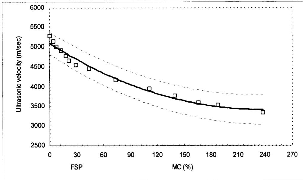
FIG. 3. Relationship between ultrasonic velocities and MC in the longitudinal direction.
