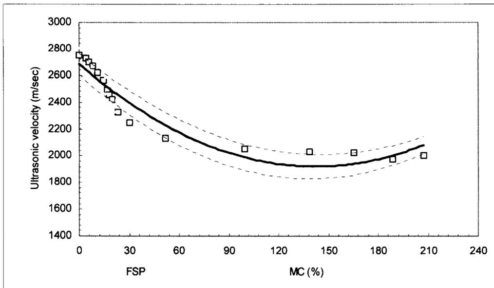
FIG. 4. Relationship between ultrasonic velocities and MC in the radial direction.
