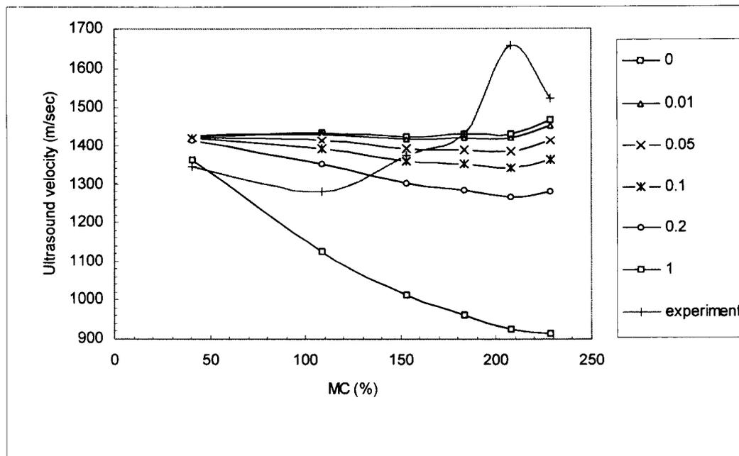
FIG. 11. Relationships between moisture content and velocity for ultrasonic wave to calculating the optimum value of the mobility of free water for tangential specimens.
