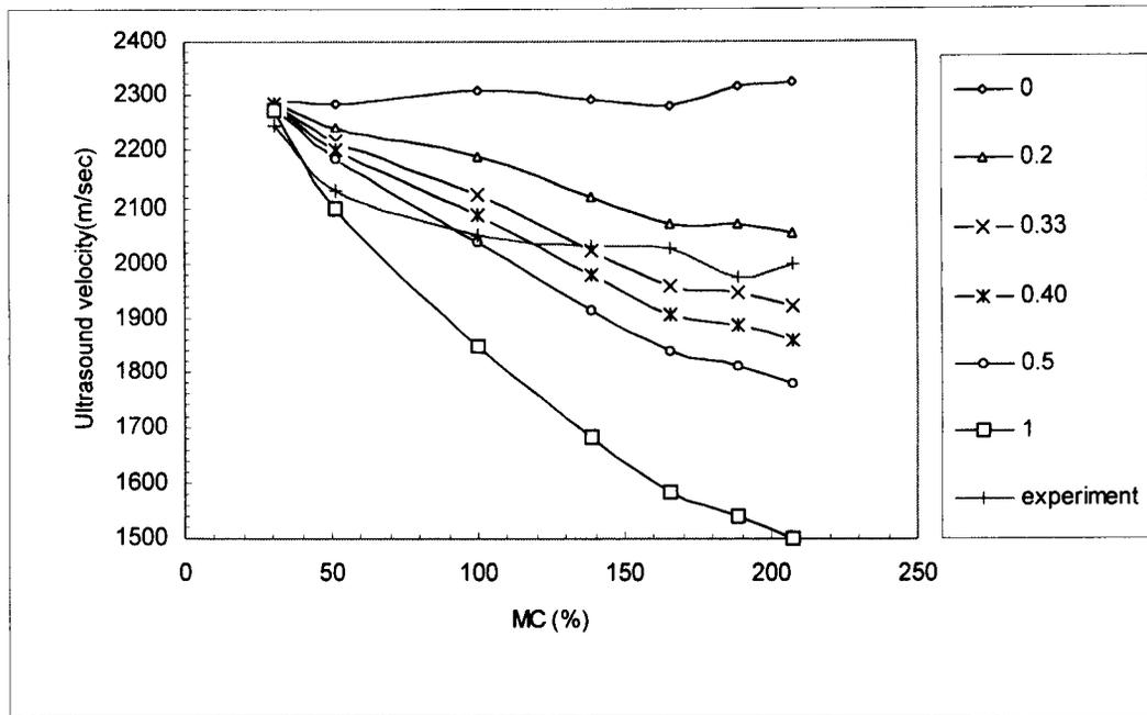
FIG. 10. Relationships between moisture content and velocity for ultrasonic wave to calculating the optimum value of the mobility of free water for radial specimens.
