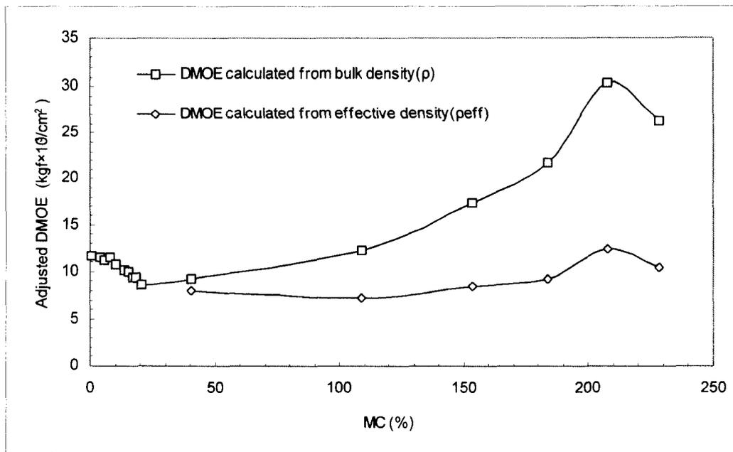
FIG. 8. Relationships between the corrected DMOE and MC in the tangential direction.
