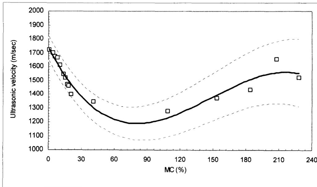
FIG. 5. Relationship between ultrasonic velocities and MC in the tangential direction.
