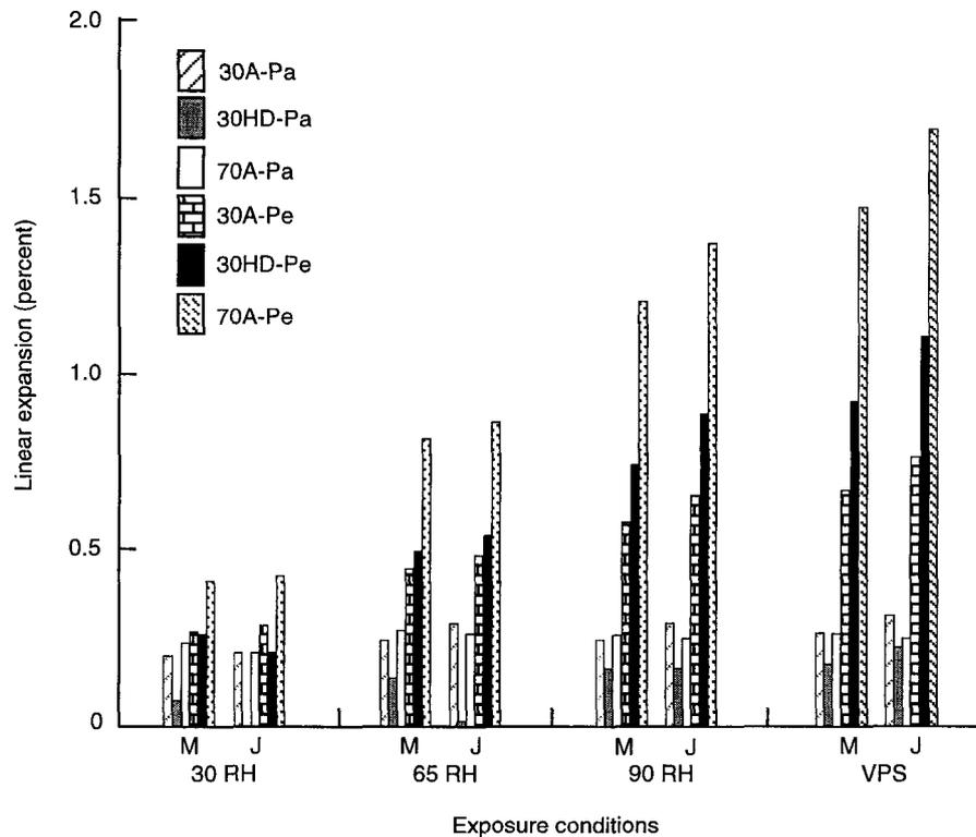
FIG. 6. Linear expansion of 30% and 70% single-layer directional flakeboard constructed with mature and juvenile wood.
