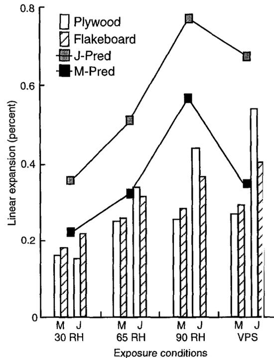
FIG. 3. Linear expansion of plywood and balanced flakeboard constructed with mature (M) and juvenile (J) wood. Values for flakeboard are averages of Pa and Pe specimens from all balanced (random, three-layer 10% cross-aligned (30XA), and 70% cross-aligned (70XA)) flakeboard. Values predicted from linear expansion and tensile modulus of veneer are shown as line graphs.
