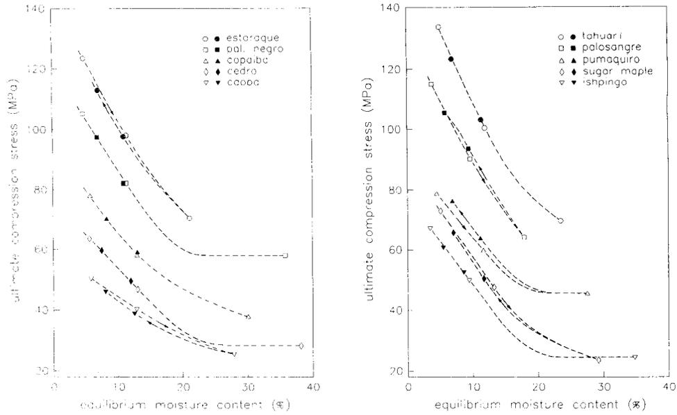
FIG. 3. Ultimate stress in parallel to grain compression ( $\sigma_{L||}$ ) for all species as a function of EMC at 25 C. Open and filled points correspond to the adsorption and desorption states respectively.
