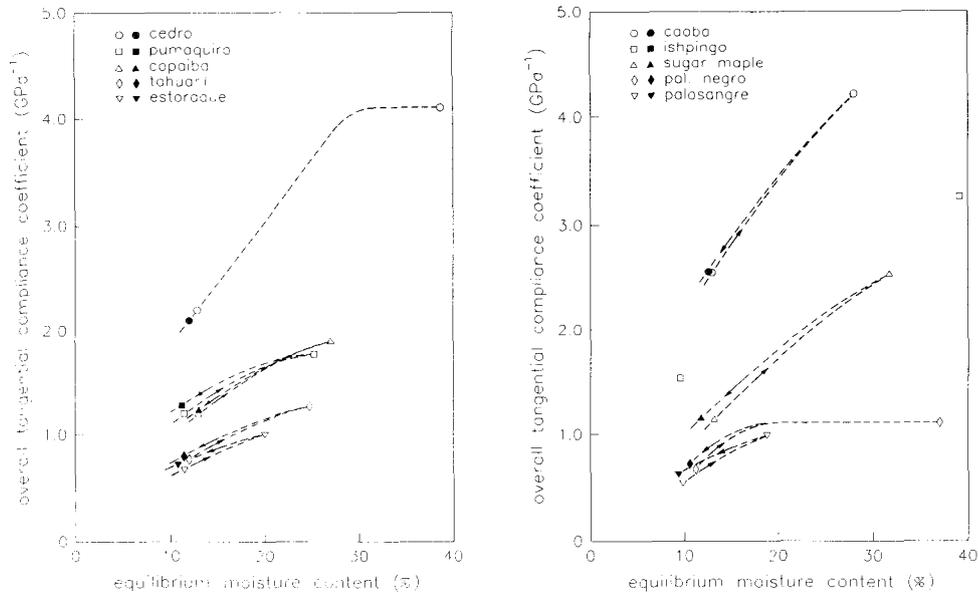
FIG. 5. Compliance coefficients  $s_{33}$  in perpendicular to grain tangential compression, measured over the entire length of specimens ( $\approx 60$  mm), for all species as a function of EMC at 25 C. Open and filled points correspond to the adsorption and desorption states respectively.
