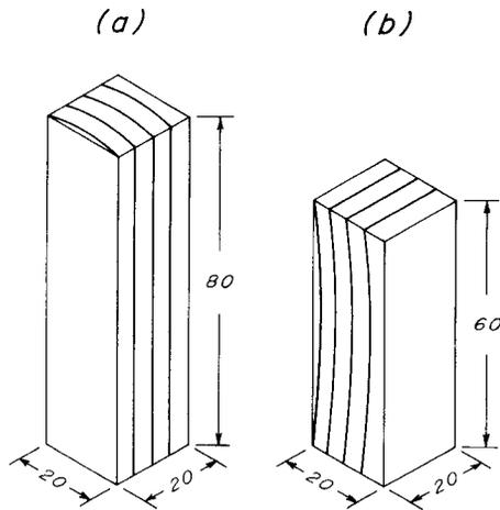
FIG. 1. Schematic representation of specimens for (a) parallel to grain compression and (b) perpendicular to grain tangential compression (mm).
