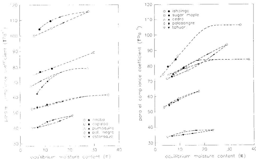
FIG. 2. Compliance coefficients  $s_{11}$  in parallel to grain compression for all species as a function of EMC at 25 C. Open and filled points correspond to the adsorption and desorption states respectively.
