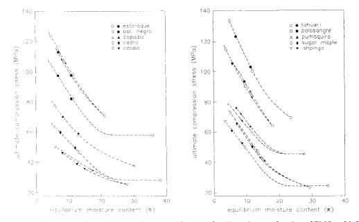
FIG. 3. Ultimate stress in parallel to grain compression ( $\sigma_{Lu}$ ) for all species as a function of EMC at 25 C. Open and filled points correspond to the adsorption and desorption states respectively.
