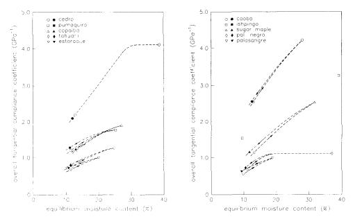
FIG. 5. Compliance coefficients  $s_{33}$  in perpendicular to grain tangential compression, measured over the entire length of specimens ( $\approx 60$  mm), for all species as a function of EMC at 25 C. Open and filled points correspond to the adsorption and desorption states respectively.
