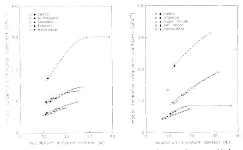
FIG. 4. Compliance coefficients  $s_{33}$  in perpendicular to grain tangential compression, measured in the central part of specimens (40 mm), for all species as a function of EMC at 25 C. Open and filled points correspond to the adsorption and desorption states respectively.
