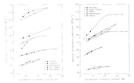
FIG. 2. Compliance coefficients  $s_{11}$  in parallel to grain compression for all species as a function of EMC at 25 C. Open and filled points correspond to the adsorption and desorption states respectively.
