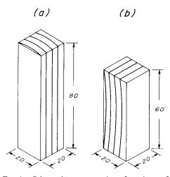
FIG. 1. Schematic representation of specimens for (a) parallel to grain compression and (b) perpendicular to grain tangential compression (mm).
