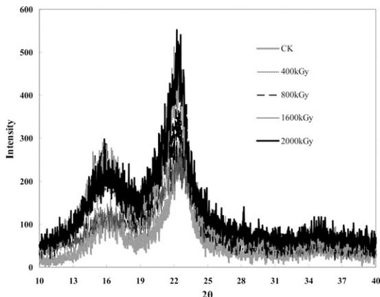
Figure 3. X-ray diffraction (XRD) images of crystalline cellulose of *Phragmites communis* trim (PCT) treated with different irradiation doses (untreated crystalline cellulose of PCT [CK]).
