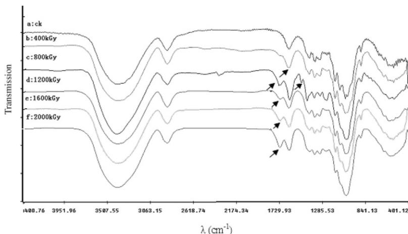
Figure 5. Fourier transform-IR spectra for the oxidative gradation of *Phragmites communis* trim (PCT) microcrystalline cellulose treated with different irradiation doses ([a] untreated microcrystalline cellulose [0 kGy]; [b] 400 kGy; [c] 800 kGy; [d] 1200 kGy; [e] 1600 kGy; [f] 2000 kGy).
