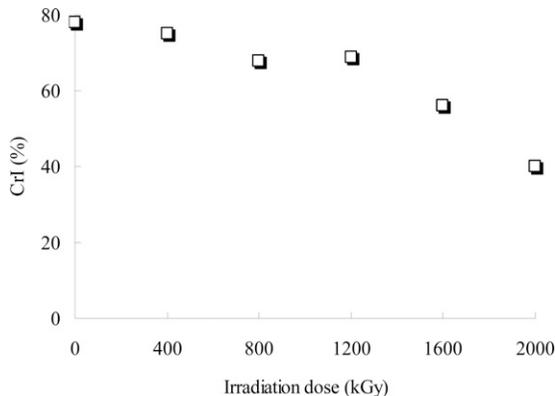
Figure 4. Variation of crystallinity index calculated from X-ray diffraction (XRD) chart.
