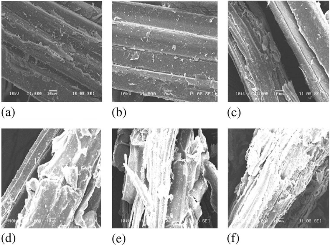
Figure 1. Scanning electron micrograph images of *Phragmites communis* trim (PCT) cellulose sample treated with different irradiation doses [(a) untreated PCT cellulose [0 kGy]; (b) 400 kGy; (c) 800 kGy; (d) 1200 kGy; (e) 1600 kGy; (f) 2000 kGy].
