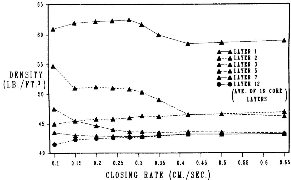
FIG. 3. Changes in density for model-predicted profile layers 1, 2, 3, 5, 7 and 12 with changes in press closing rate.
