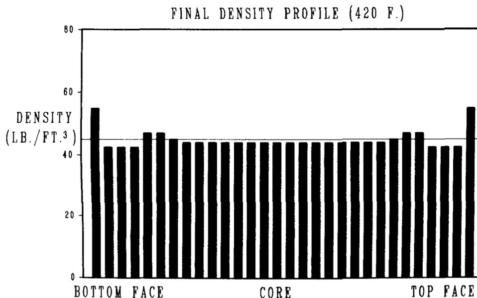
FIG. 4. Model-predicted density profile resulting from an uneven initial moisture distribution.
