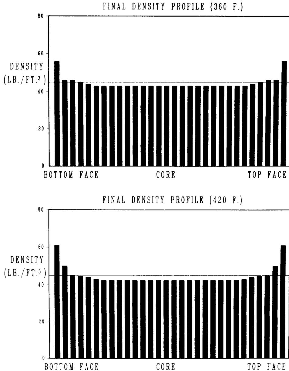
FIG. 2. Model-predicted density profiles for platen temperatures 360 F and 420 F.
