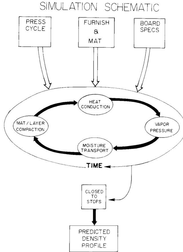
FIG. 1. Schematic of user inputs and simulation.
