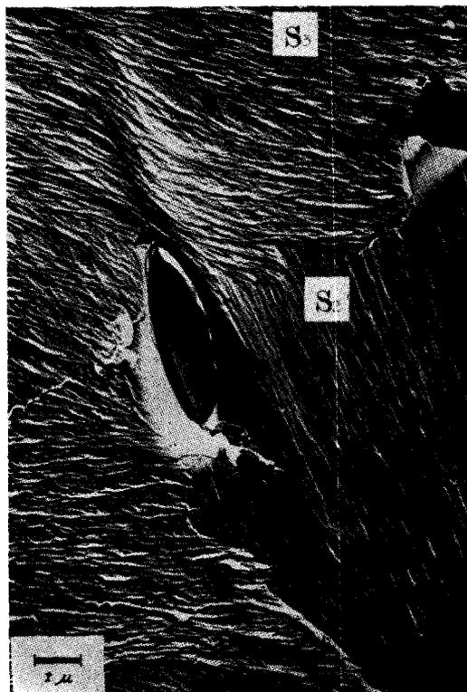
FIG. 9. Microfibrillar orientation in the S2 layer and the overlying S3 layer as viewed from the inner surface of an earlywood tracheid of spruce (Harada 1958).
