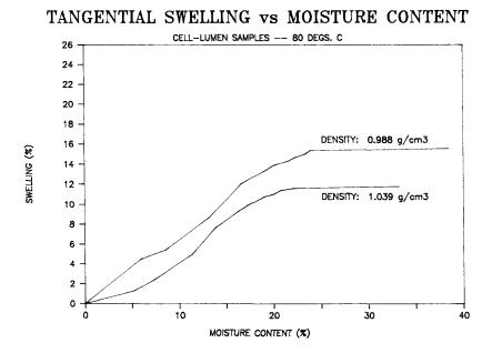
FIG. 3. Swelling of different density cell lumen wood polymer composite samples in 80 C water. Fiber saturation point appears to be 20% MC for the higher density sample and 25% MC for the lower density sample.
