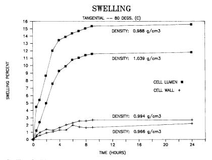
FIG. 2. Swelling of cell lumen and cell-wall wood polymer composite samples in hot (80 C) water.
