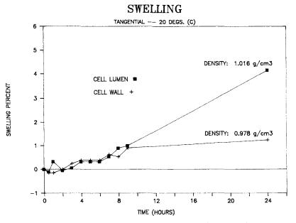
FIG. 1. Swelling of cell lumen and cell-wall wood polymer composite samples in room temperature water.
