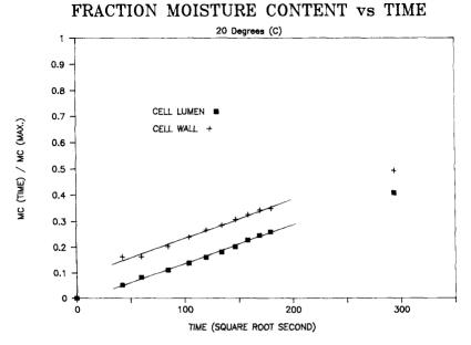
FIG. 5. Fraction of maximum MC vs. time for cell lumen and cell-wall wood polymer composite samples in room temperature water. Lines are linear regressions.
