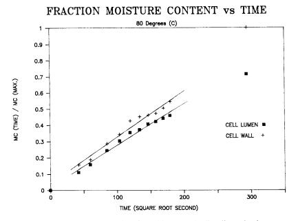
FIG. 6. Fraction of maximum MC vs. time for cell lumen and cell-wall wood polymer composite samples in hot (80 C) water. Lines are linear regressions.
