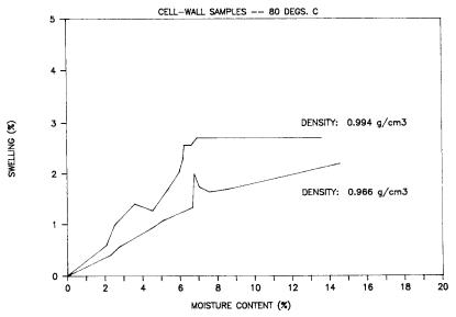
FIG. 4. Swelling of different density cell-wall wood polymer composite samples in 80 C water. Fiber saturation point appears to be 8% MC.
