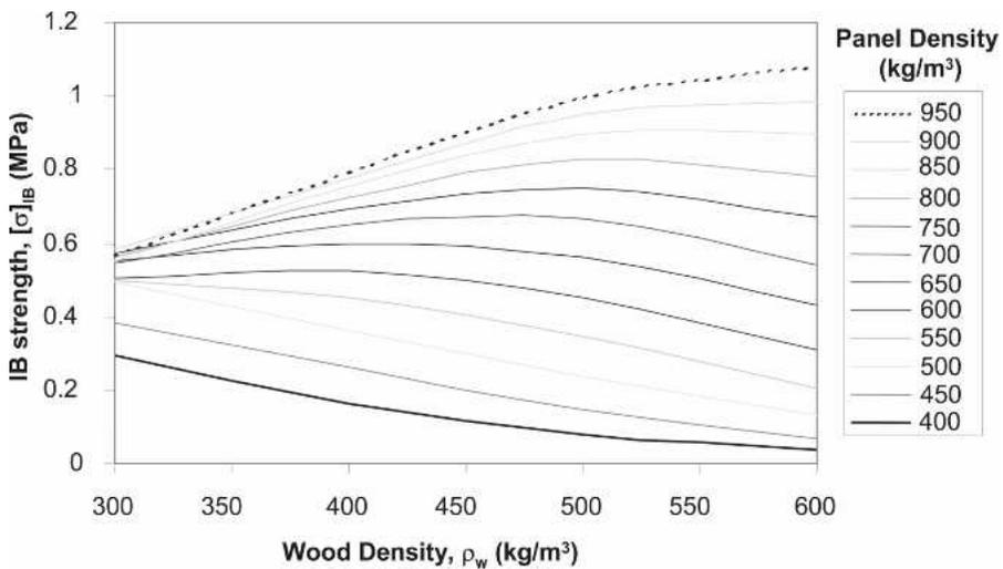
FIGURE 12. Predicted effects of wood density on the IB strength at various panel densities.
