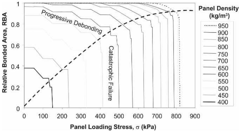
FIGURE 9. Predicted changes of relative bonded areas during debonding and catastrophic failure processes (the values are in steps of 50 from 400–950 kg/m<sup>3</sup> from left to right).
