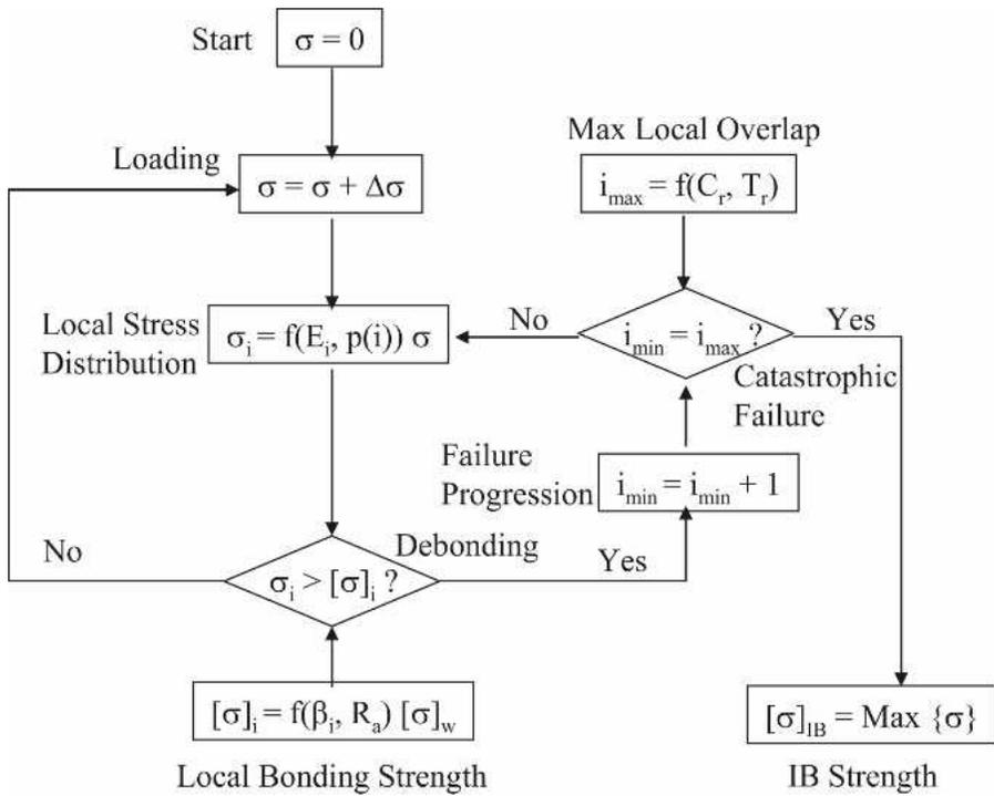
FIGURE 2. Flowchart of the computer model showing the logics of IB calculation.
