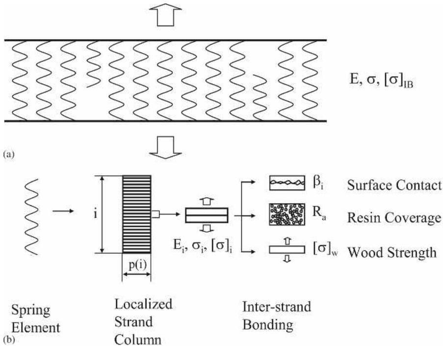
FIGURE 1. Schematic of the IB model. (a). A parallel spring-field model, and (b). Linkage between localized column of bonded strands, surface contact, resin coverage, and wood strength. Note that  $i$  is both the index counter and the overlap number of a column.
