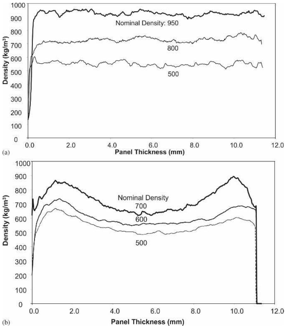
FIGURE 3. Vertical density profiles of laboratory-made strandboards. (a). Specially pressed uniform density profiles, and (b). Conventional vertical density profiles.
