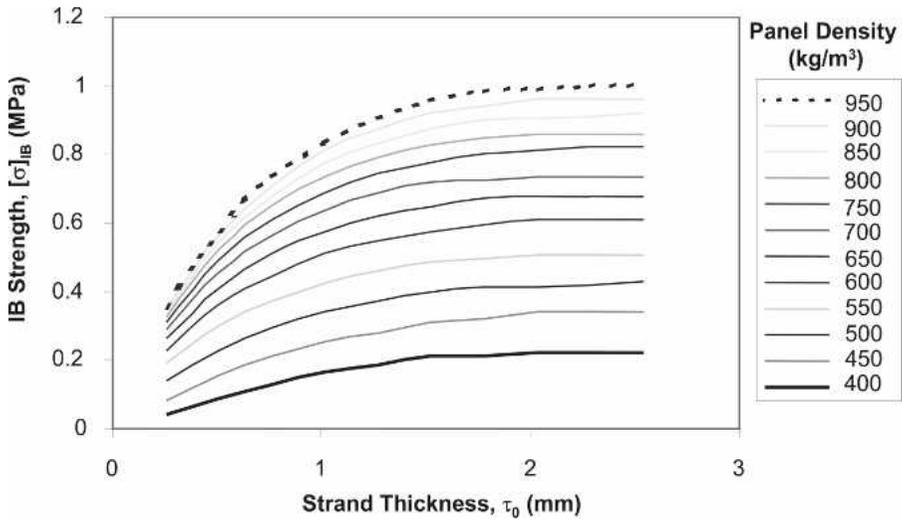
FIGURE 11. Predicted effects of strand thickness on the IB strength at various panel densities.
