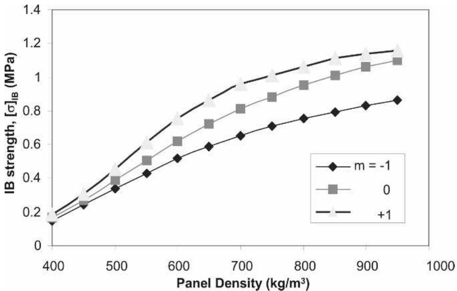
FIGURE 7. Predicted effect of strand softening index on the IB strength.
