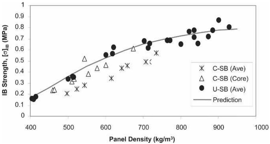
FIGURE 4. Comparing IB strengths between the model predictions and the experimental data.
