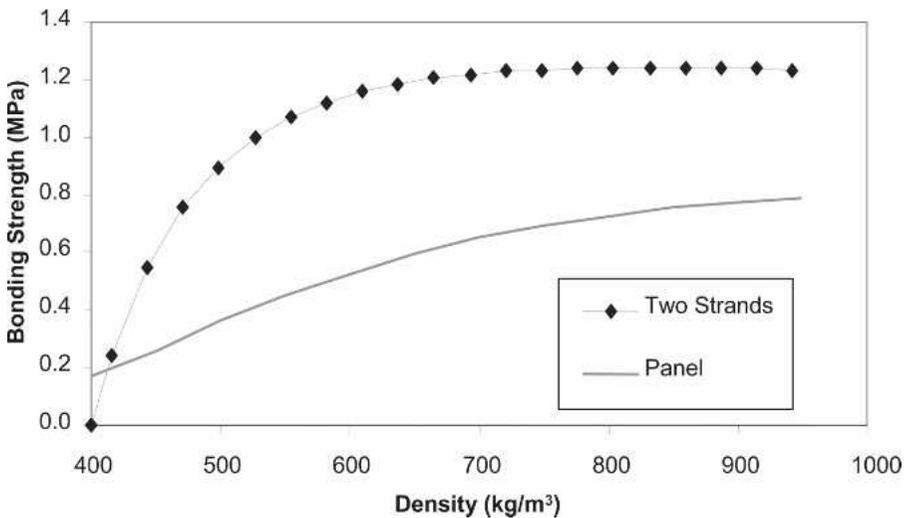
FIGURE 5. Comparing bonding strengths between two overlapped strands and regular strandboards.
