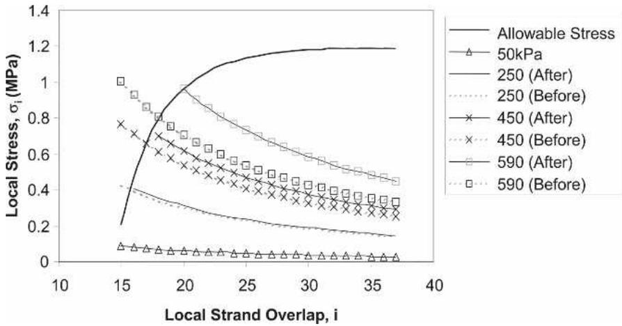
FIGURE 8. Predicted stress redistributions due to localized bond failures.
