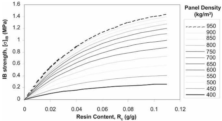
FIGURE 10. Predicted effects of resin content on the IB strength at various panel densities.
