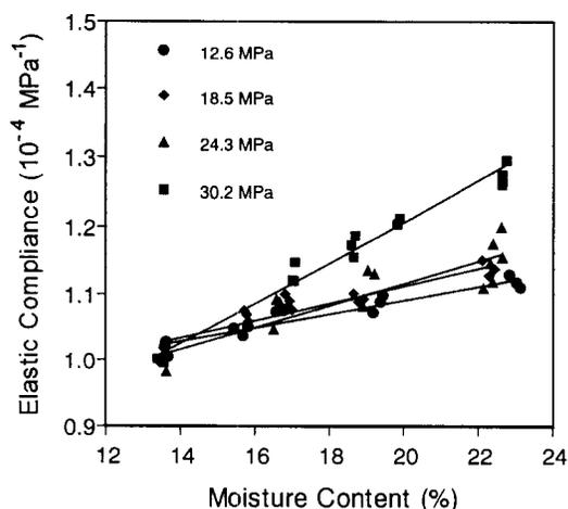
FIG. 2. Elastic compliance as a function of moisture content at four stress levels, showing results of a linear fit.
