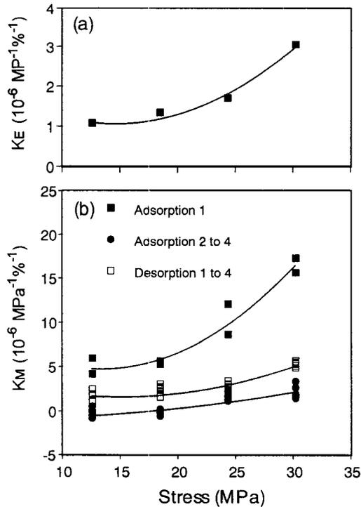
FIG. 4. Elastic parameter  $K_E$  (a) and MS parameter  $K_M$  (b) as a function of applied stress.
