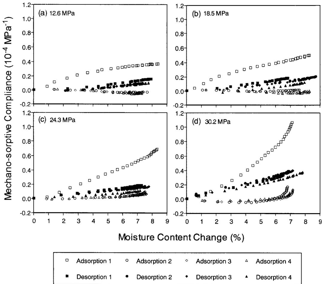
FIG. 3. The relationship between mechano-sorptive compliance and moisture content change at four stress levels.
