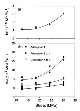
FIG. 4. Elastic parameter  $K_{\rm E}$  (a) and MS parameter  $K_{\rm M}$  (b) as a function of applied stress.
