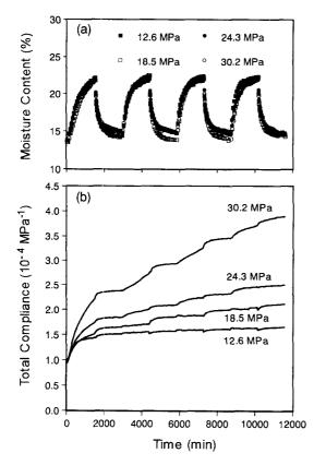
FIG. 1. Moisture content change (a) and total compliance (b) as a function of sorption time at four stress levels.
