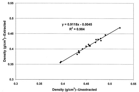
Fig. 2. Simple linear regression with plotted overall mean density values for extracted vs. unextracted samples.
