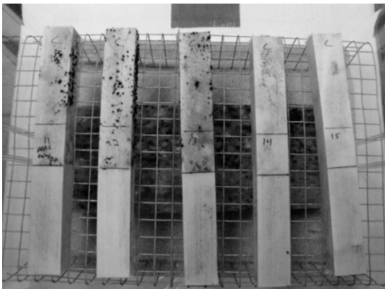
Figure 2. Example of sweetgum test samples after cycle 1.
