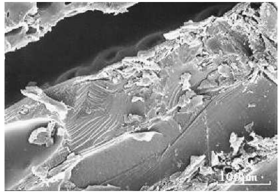
FIGURE 11. PF resin in lumen by SEM.
