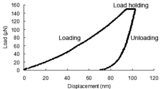
Figure 3. Representative nanoindentation load-displacement curve drawn from a result of nanoindentation.
