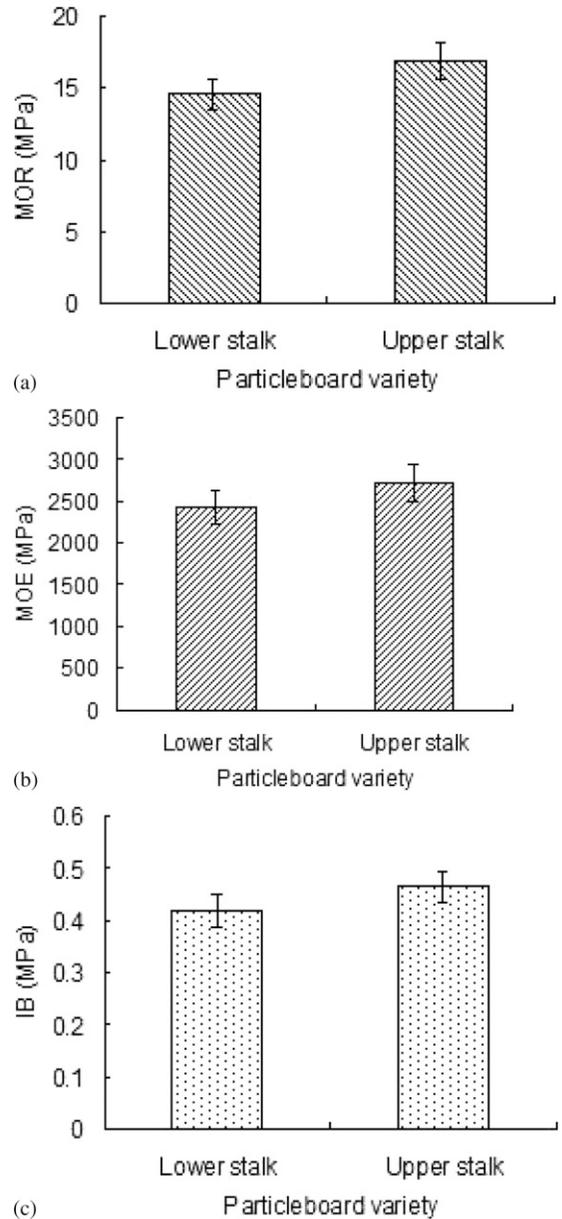
Figure 4. Mechanical properties of particleboard made from silvergrass stalk: (a) modulus of rupture (MOR); (b) modulus of elasticity (MOE); (c) internal bond strength (IB).
