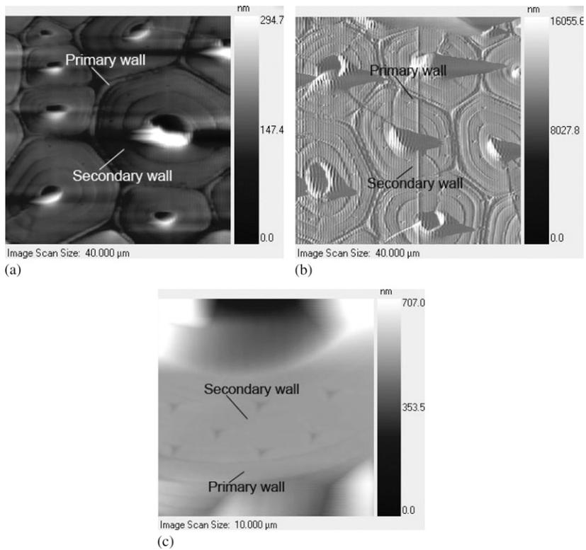
Figure 2. Scanning probe microscopy (SPM) images of silvergrass fibers and parenchyma cell: (a) nanoscale structure of silvergrass fiber cells; (b) indentations on silvergrass fiber cell walls; (c) SPM image of silvergrass parenchyma cell in upper stalk.
