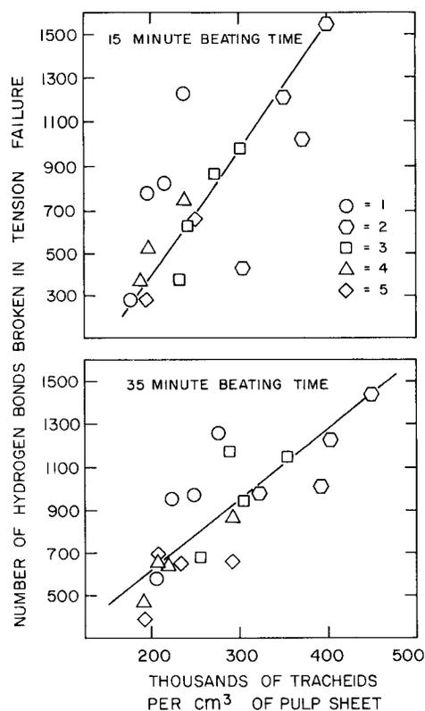
FIG. 7. The influence of the number of tracheids per unit volume, fractions (1-5) and beating time (15 and 35 min) on the number of hydrogen bonds broken in paper sheets in tension.
