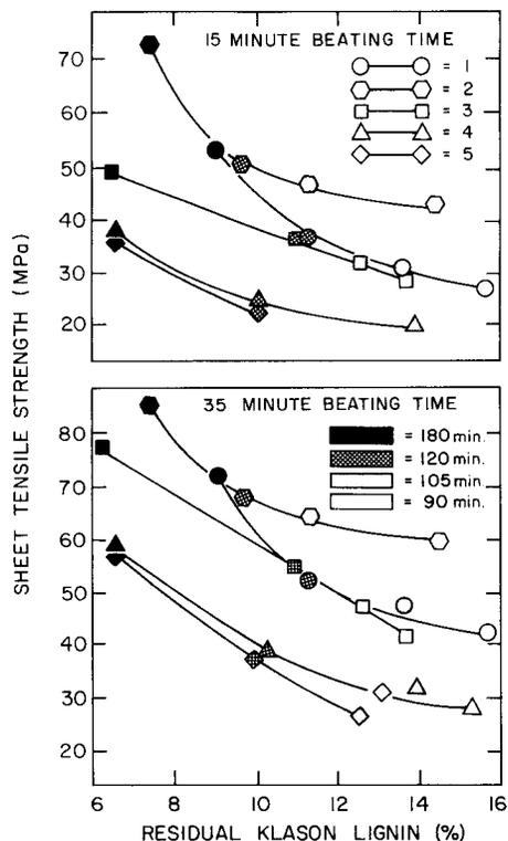
FIG. 3. The influence of residual Klason lignin on the tensile strength of pulp sheets from five incremental growth zones (1-5) following four digestion times (90-180 min) and two beating periods (15 and 35 min).
