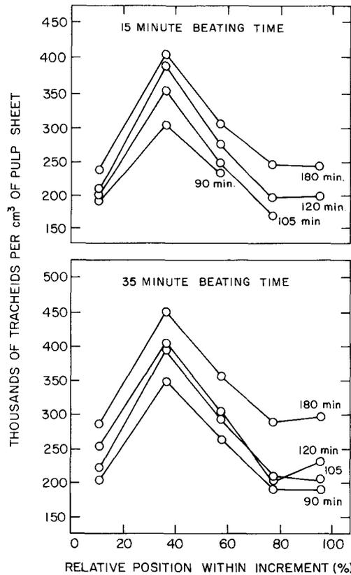
FIG. 1. Number of tracheids per unit volume of pulp sheet as a function of within-growth-ring source, kraft digestion times of 90, 105, 120, and 180 min, and beating times of 15 and 35 min.
