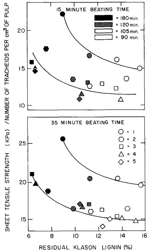
FIG. 4. Influence of residual Klason lignin, intraincrement fraction (1-5), and beating time (15 and 35 min) on the contribution of individual tracheids to sheet tensile strength after four cooking times (90-180 min.).
