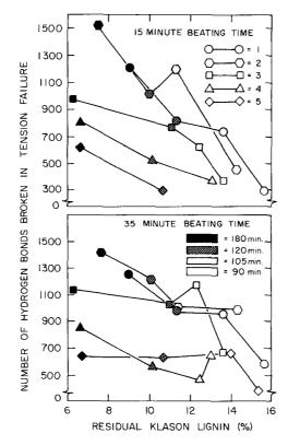
FIG. 6. Hypothetical number of hydrogen bonds broken in paper sheets in tension as a function of residual Klason lignin and beating times (15 and 35 min) for the five fractions and four digestion times (90–180 min).
