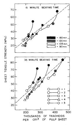
FIG. 2. Relationship between sheet tensile strength and number of tracheids per unit volume of pulp sheet after two beating periods (15 and 35 min) for five intraincrement fractions (1–5) after four cooking times (90–180 min).
