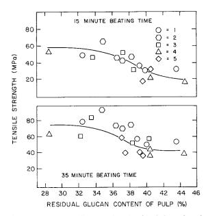
FIG. 5. Relationship between sheet tensile strength and residual glucan in pulps from five intraincrement fractions at two beating times (15 and 35 min).
