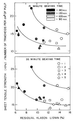
FIG. 4. Influence of residual Klason lignin, intraincrement fraction (1-5), and beating time (15 and 35 min) on the contribution of individual tracheids to sheet tensile strength after four cooking times (90-180 min.).
