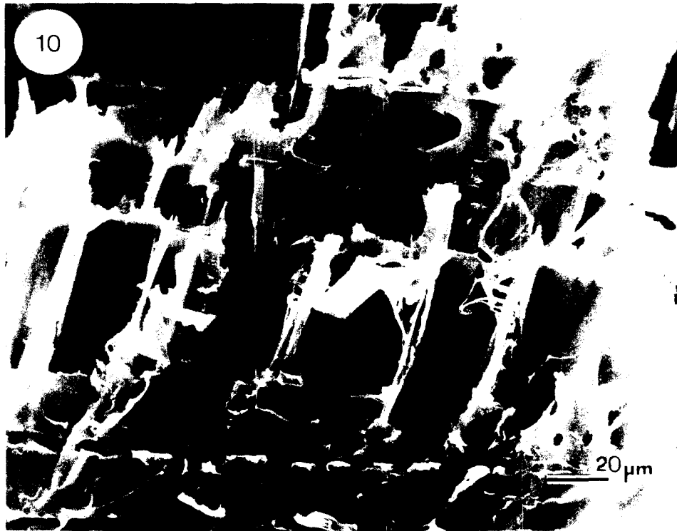
FIG. 10. Scanning electron fractograph of a longitudinal-radial fracture plane in wood decayed by Trametes versicolor to 2% weight loss. The step angles of failure across the longitudinally oriented cells were steep just like that of sound wood.
