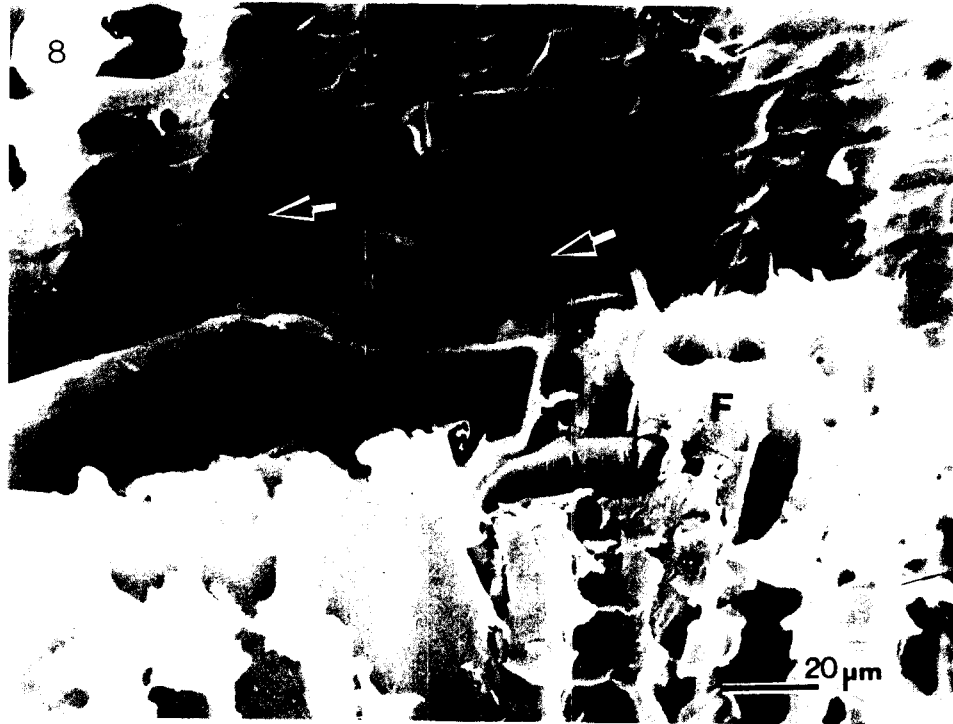
FIG. 8. Scanning electron fractograph showing a longitudinal-radial fracture plane in wood decayed by Bjerkandera adusta to 10% weight loss. Observe how the ray cell (R) was degraded (arrows) and how abrupt transwall fracture (tw) of vessels (V) and fibers (F) occurred at angles almost perpendicular to the grain direction.
