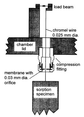
FIG. 2. Schematic drawing of weighing mechanism for the pressurized sorption apparatus.
