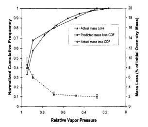
FIG. 8. Mass loss due to wood degradation as a function of relative vapor pressure, for desorption of mature yellow-poplar at 160°C. Lines represent normalized mass loss in the form of a cumulative distribution function (CDF).
