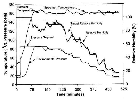
FIG. 3. Environmental conditions and specimen temperature for a desorption experiment at 160°C.
