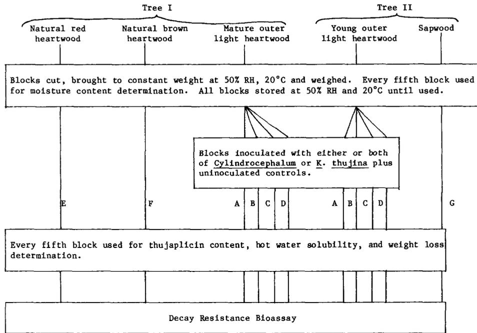
FIG. 1. Flow chart of methods showing the origin of test blocks and the sequence of measurements and treatments.
