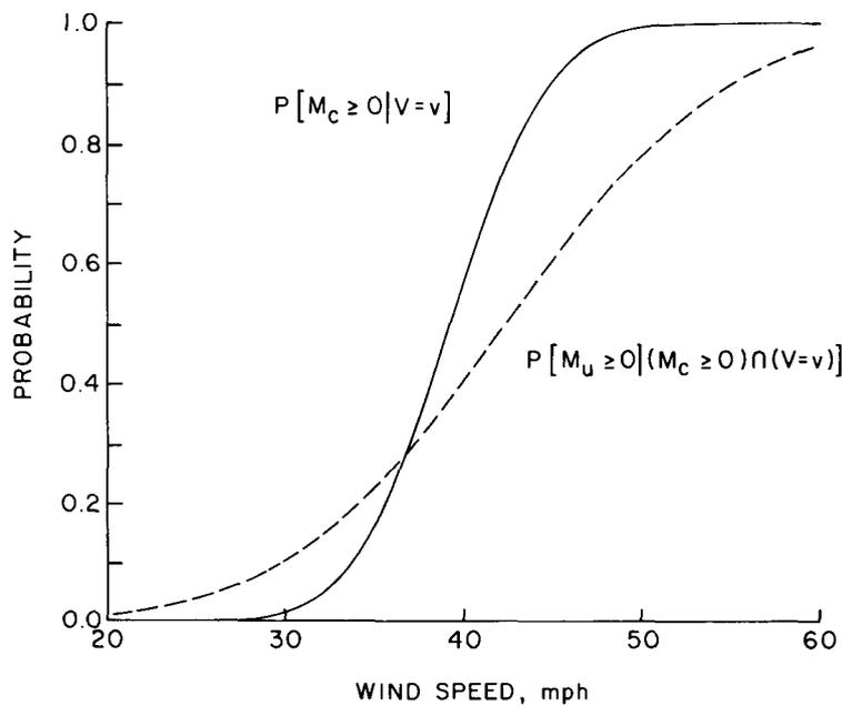
FIG. 6. Conditional probabilities for tree cracking and collapse, case 1.
