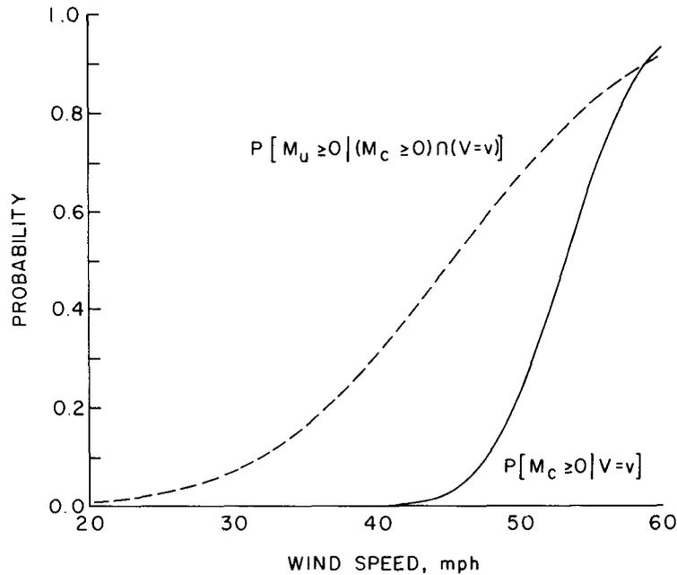
FIG. 7. Conditional probabilities for tree cracking and collapse, case 2.
