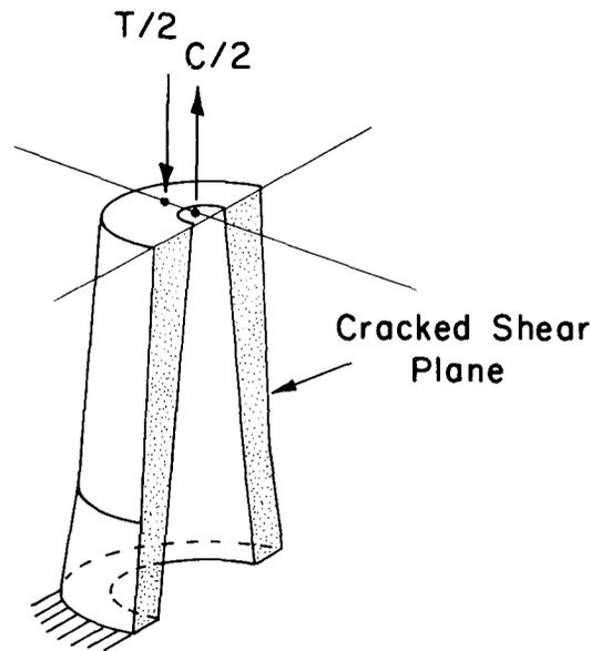
FIG. 4. The collapse phase.
