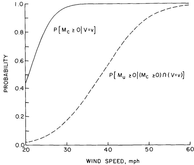
FIG. 8. Conditional probabilities for tree cracking and collapse, case 3.
