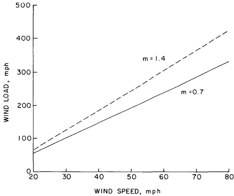
FIG. 9. The effect of moisture content on wind loading.
