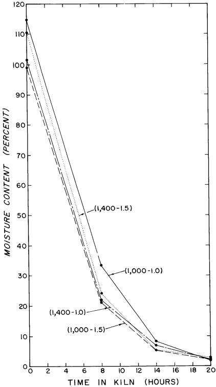
F1G. 1. Changes in moisture content in 4- and 6-inch wide, 1.75-inch-thick southern pine lumber dried in 5-ft-wide loads at 260 F (wet-bulb temperature was 180 F) after 8, 14, and 20 h of kiln time (including 434 h of kiln warmup time), with air cross-circulation velocities of 1,000 and 1,400 fpm and stick thicknesses of 1.0 and 1.5 inches.
