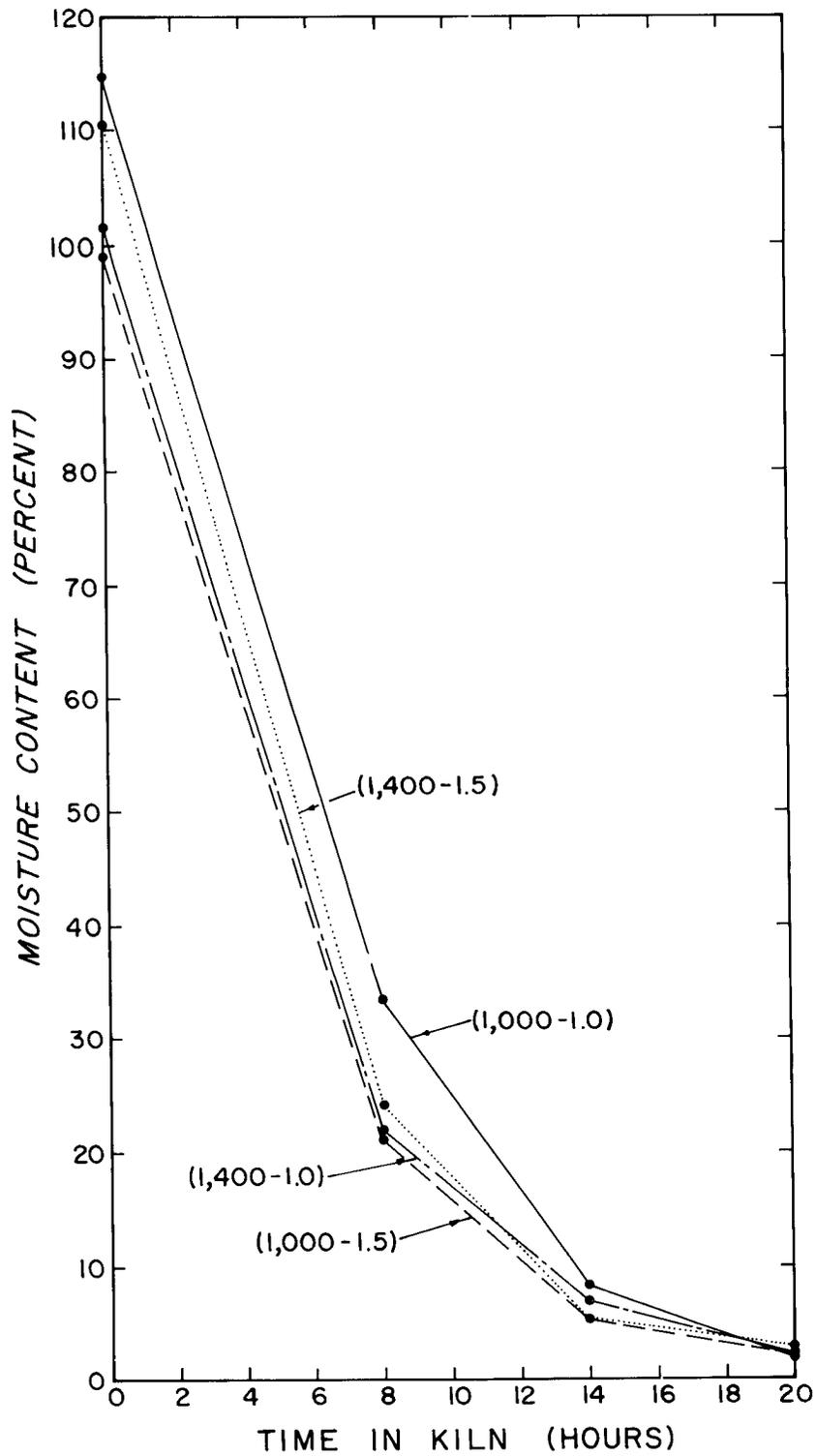
FIG. 1. Changes in moisture content in 4- and 6-inch wide, 1.75-inch-thick southern pine lumber dried in 5-ft-wide loads at 260 F (wet-bulb temperature was 180 F) after 8, 14, and 20 h of kiln time (including 4¾ h of kiln warmup time), with air cross-circulation velocities of 1,000 and 1,400 fpm and stick thicknesses of 1.0 and 1.5 inches.
