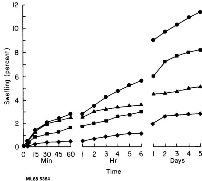
FIG. 1. Rate of thickness swelling of veneer-faced low-density particleboards in liquid water. ● control veneers, control particles; ■ acetylated veneers, control particles; ▲ control veneers, acetylated particles; ◆ acetylated veneers, acetylated particles.
