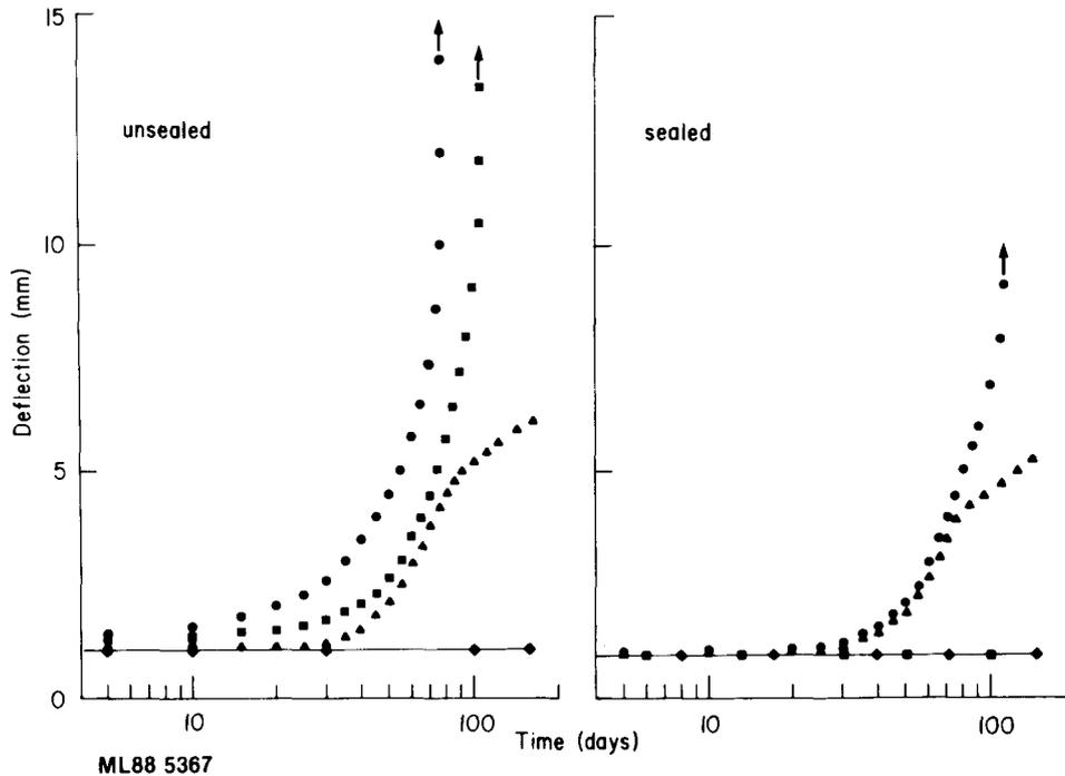
FIG. 4. Deflection time curves of unsealed and sealed veneer-faced low-density particleboards under progressive fungal attack by *T. palustris* on bending-creep test. ● control veneers, control particles; ■ acetylated veneers, control particles; ▲ control veneers, acetylated particles; ◆ acetylated veneers, acetylated particles.
