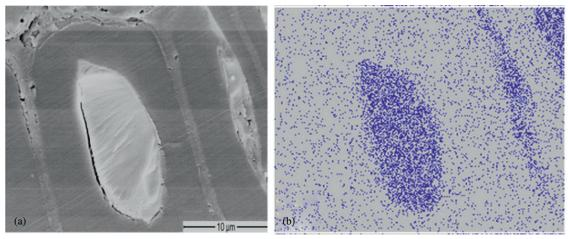
Figure 7. Cross-sectional view of Douglas-fir specimen bonded with high molecular weight iodinated phenol formaldehyde, never exposed to weathering; (a) scanning electron microscope, scale bar is  $10 \ \mu m$  and (b) same view showing elemental map of iodine.
