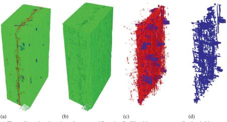
Figure 3. (a) Three-dimensional section of segmented Douglas-fir. Wood is green, pure adhesive is blue, wood–adhesive mix is red. Low contrast between the background and the wood leads to ring artifacts as seen in the bottom of this section. (b) Only the wood cells. (c) Only pure adhesive and wood–adhesive mix. (d) Only pure adhesive.
