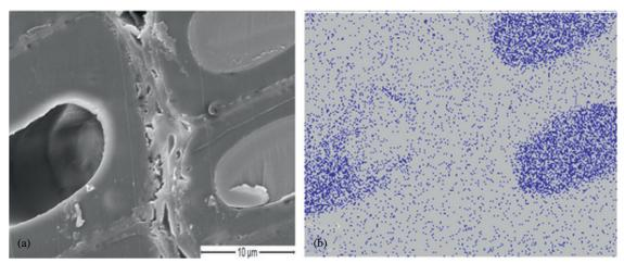
Figure 6. Cross-sectional view of Douglas-fir specimen bonded with iodinated polymeric methylene diphenyl diisocyanate (IpMDI), exposed to weathering; (a) scanning electron microscope, scale bar is 10 µm and (b) same view showing elemental map of iodine.
