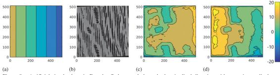
Figure 9. Artificial simple shear in Douglas-fir latewood along the longitudinal direction with a maximum displacement of  $\pm 12$  pixels; (a) applied displacement field, (b) slice from the input volume, (c) absolute difference between the applied displacement field and the calculated field from digital volume correlation (DVC), and (d) results of DVC for the slice.
