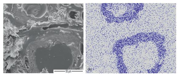
Figure 5. Cross-sectional view of Douglas-fir sample bonded with low molecular weight iodinated phenol formaldehyde, exposed to weathering (this section has a lot of cell wall tear-out but two large lumens lined with adhesive can still be distinguished); (a) scanning electron microscope, scale bar is  $50 \,\mu\text{m}$  and (b) same view showing elemental map of iodine.
