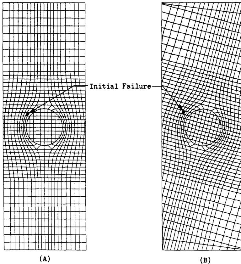
FIG. 2. Program STARWX predicted initial failure to occur due to shear stress at the location indicated.
