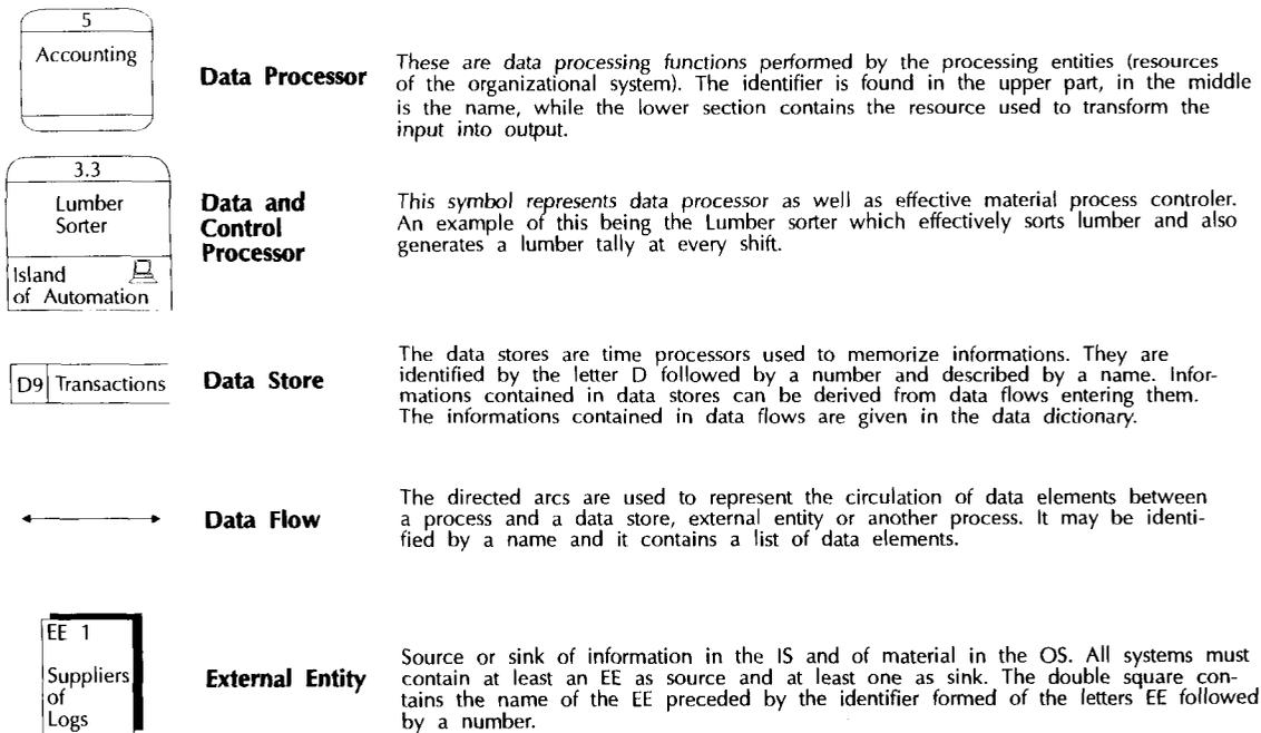
FIG. 2. Pictograms used in the Data Flow Diagrams (adapted from Mantha et al. 1988).
