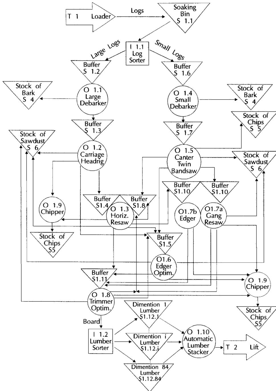
FIG. 5. Expanded view of the sawmill processor (O 1).
