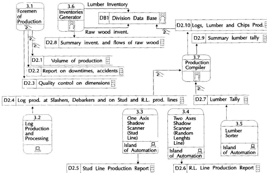
FIG. 10. Integrated Sawmill: Expanded view of the Processor 3: Produce Lumber.
