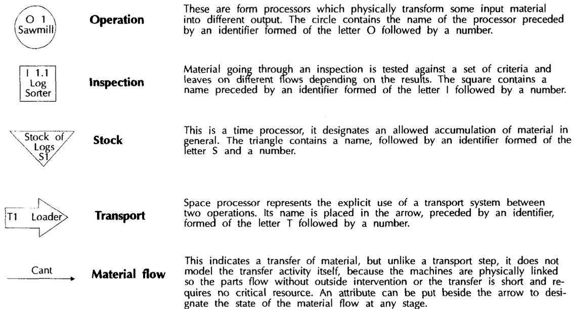
FIG. 1. Pictograms used in the Material Flow Networks (adapted from Salvendy 1982).
