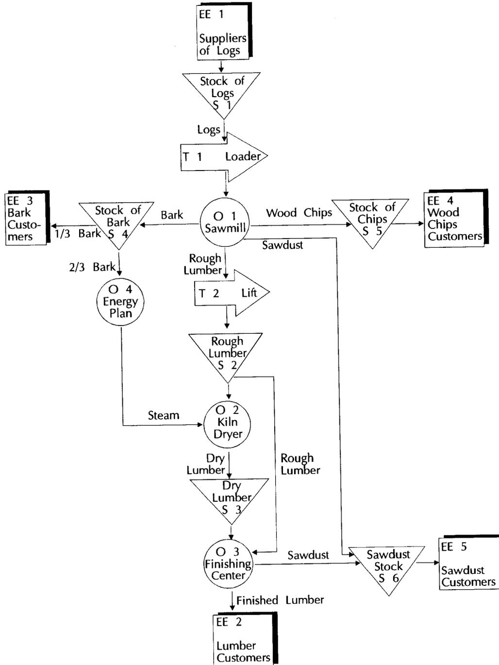
FIG. 4. A view of the Operating System of the Independent Sawmill: The context diagram of the Material Flow Network.
