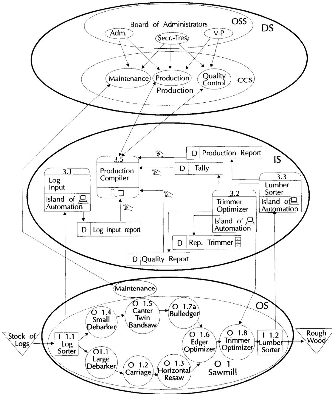
FIG. 8. Expanded view of the Production Subsystem.
