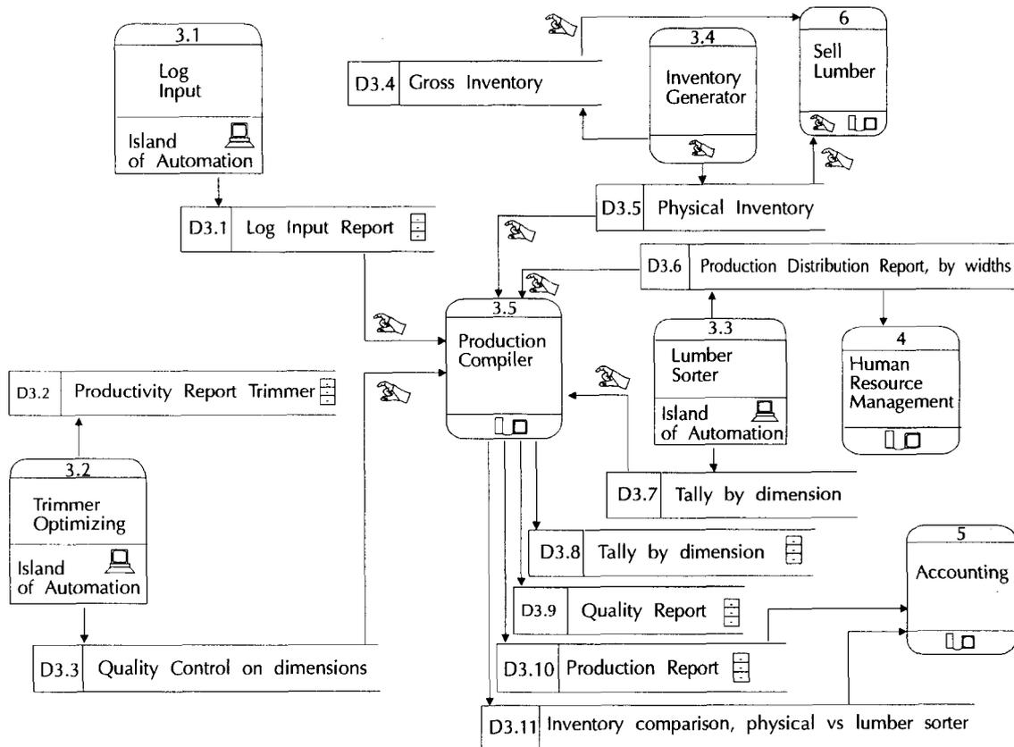
FIG. 7. Independent Sawmill: Expanded view of the Processor 3: Produce Lumber.
