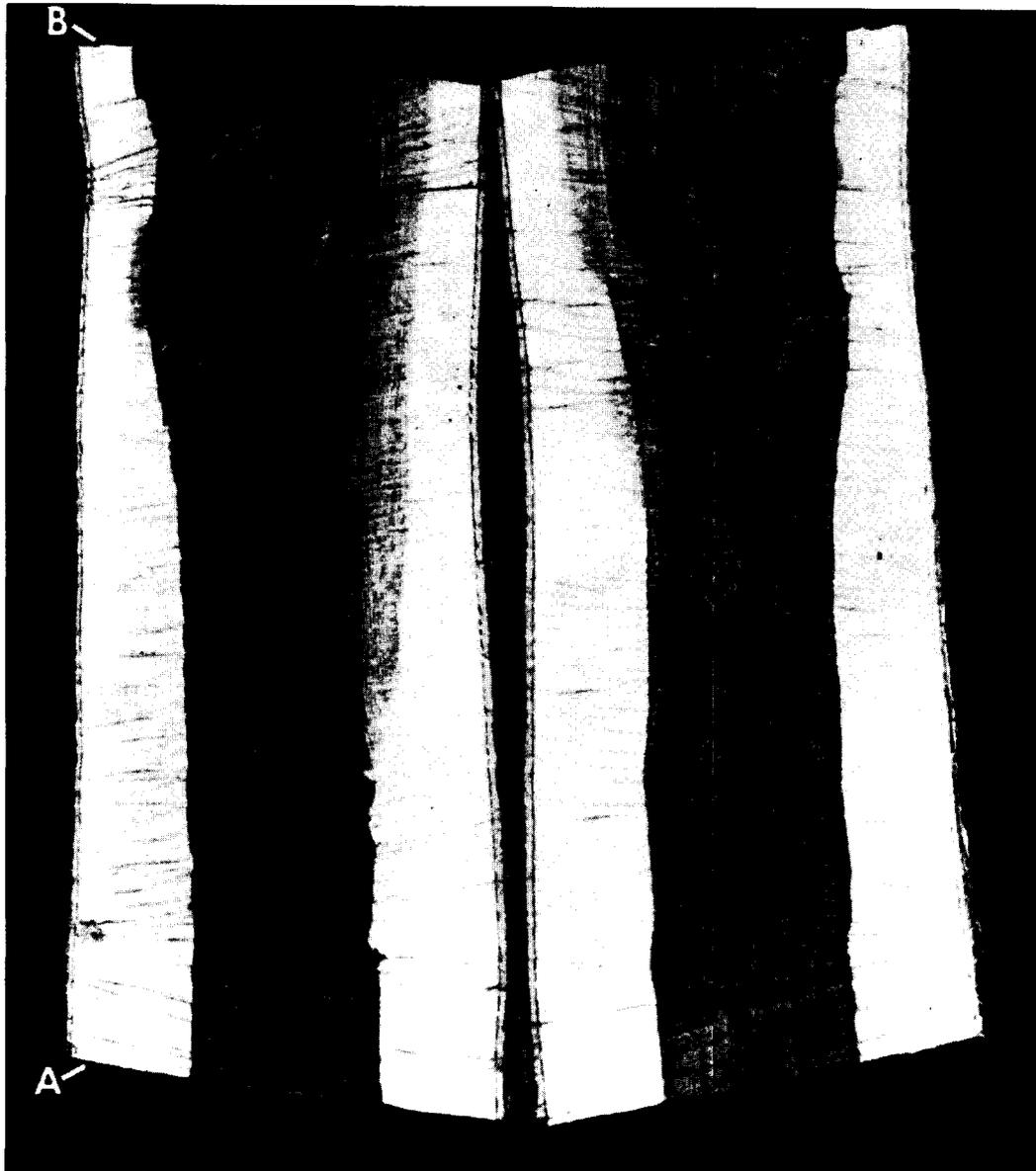
FIG. 3. Dissection of white oak sample (fire-wounded tree) from Maine showing central column of decay surrounded by 23 rings of sapwood at A, and 9 rings of sapwood only 1 m higher at B.
